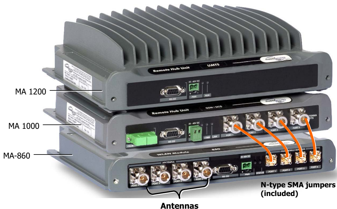
Figure 4-4. Connection of MA-860 and MA 1000 Service Ports
