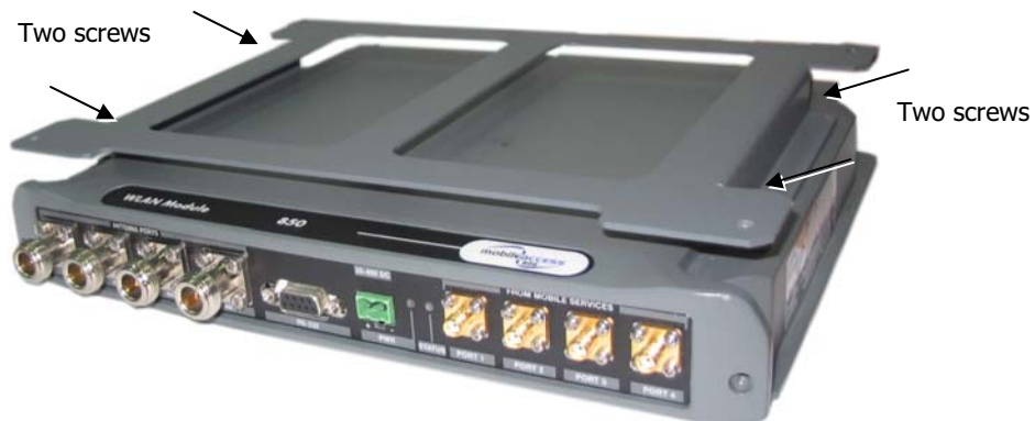
Figure 4-3. MA-860 and Bracket Assembly
