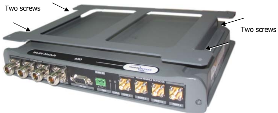
Figure 4-2. MA-860 and Bracket Assembly
