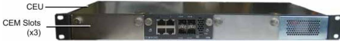
Figure 3-2. CEU Front Panel with Installed CEM Module
