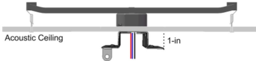
Figure 6-9: Below Ceiling Installation
