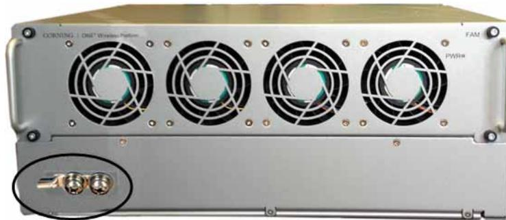
Figure 5-29. OIU Grounding Lug (Chassis Rear)
