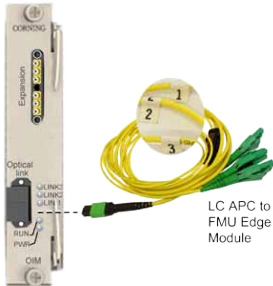
Figure 5-30. OIM Fiber Connections
