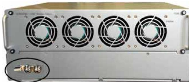
Figure 5-8. Grounding lug (HEU Chassis Rear)
