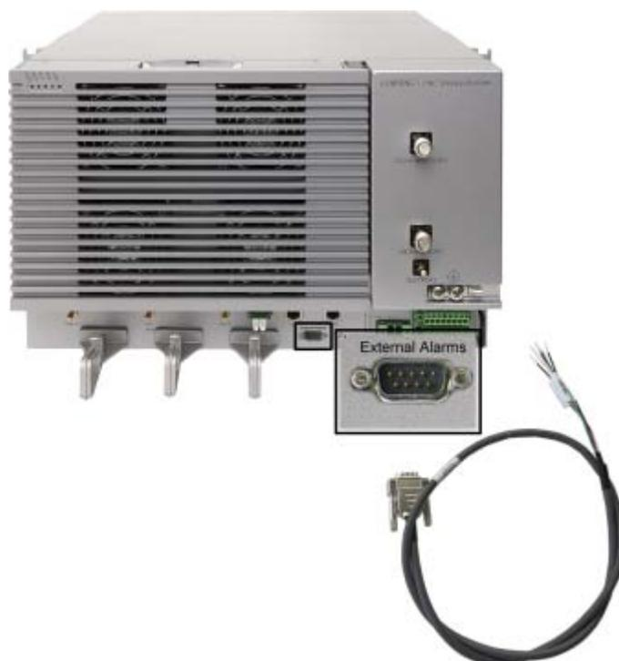
Figure 4-17. MRU External Alarms Connector and Cable
