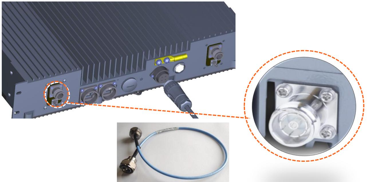
Figure 94. Antenna Connection
