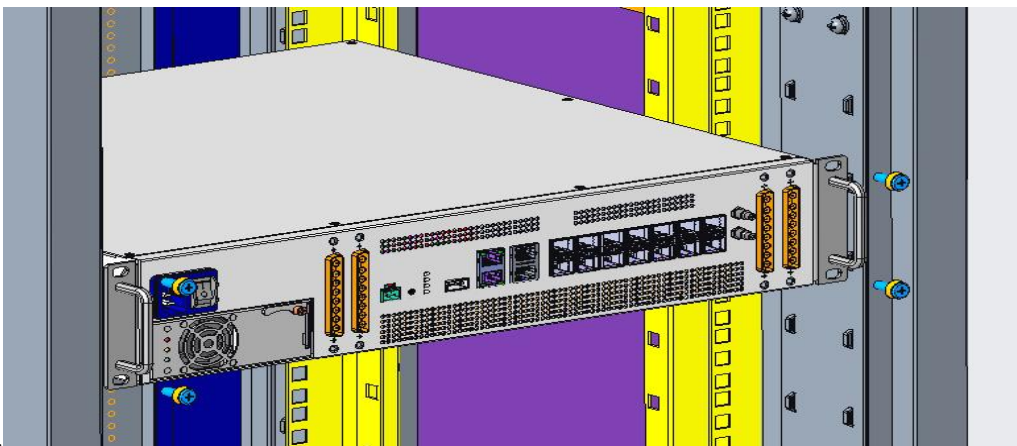
Figure 36. Installation Diagram of DCU in the Rack
