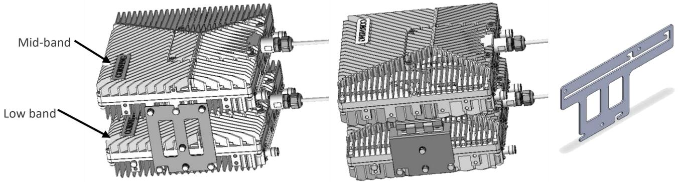
**Note: Ensure the Low Band dRAU device is connected at the bottom, and the mid-band on top!**
