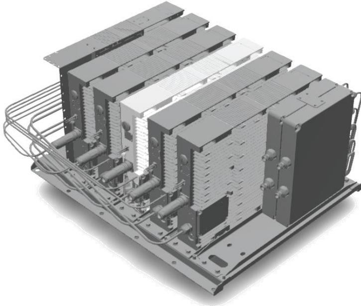
The HRU is a high power modular remote antenna unit which provides 43 dBm output RF power per service module, and native support of 2x2 MIMO antenna scheme. The HRU modular structure enables set ups of up to 8 service modules in 600/700 MHz Low/700 MHz High/FirstNet, 800/850 MHz, EAWS, PCS, WCS and 2.5GHz TDD.
