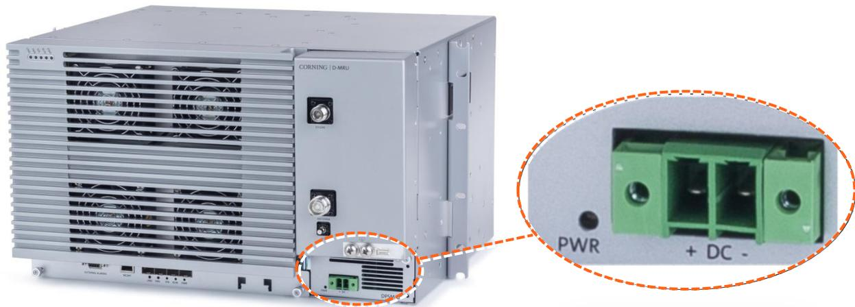
1. Open PSM captive screws and pull out module from chassis.
