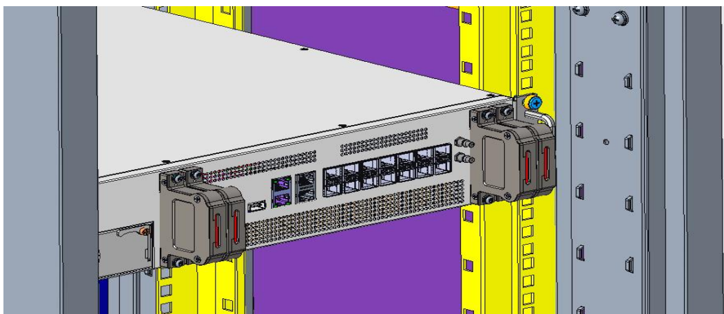
Figure 31 DCU RF cable plug installation
