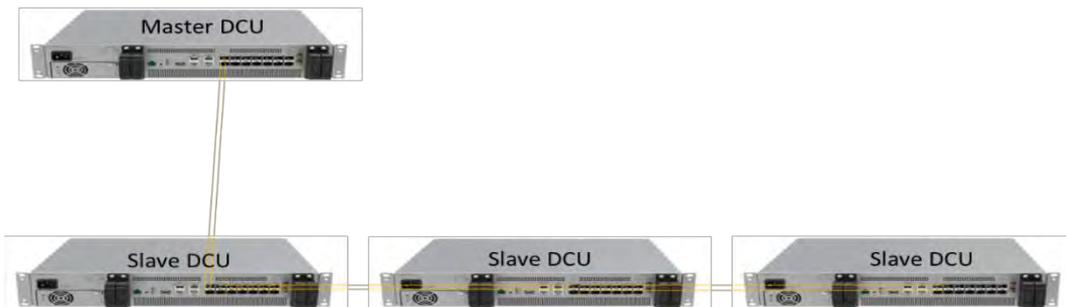
Figure 11. DCU Daisy Connection
