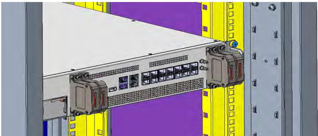
Figure 31 DCU RF cable plug installation
