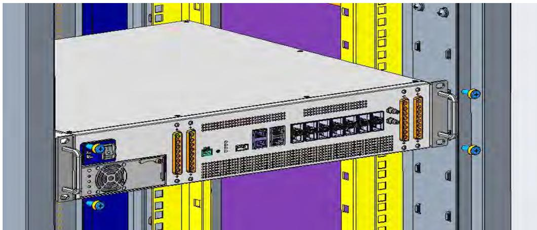
Figure 30 Installation diagram of DCU in the Rack
