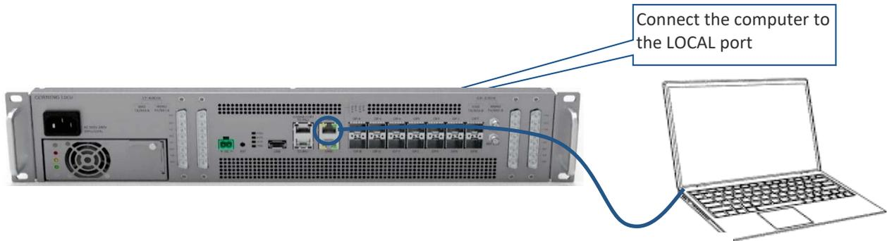
Figure 75. GUI Connection
