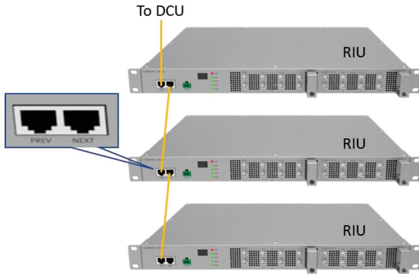
Figure 6. RIU Monitoring Diagram
