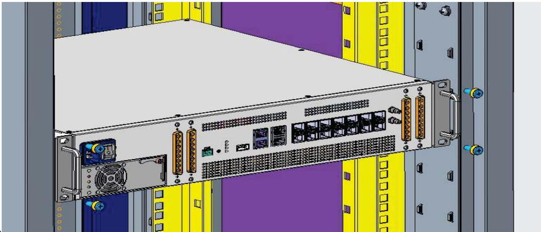
Figure 29. Installation Diagram of DCU in the Rack
