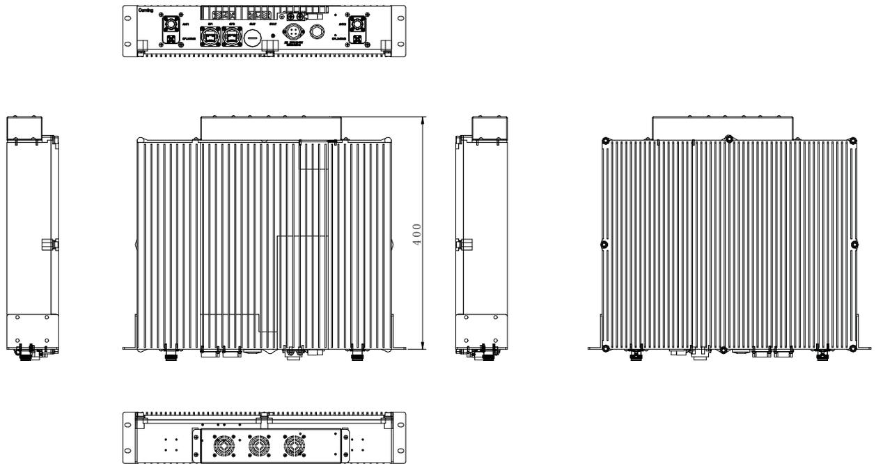
Figure 62. DMRU Dimensions - with Fan
