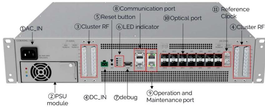
Figure 12. DCU Interface (front view)
