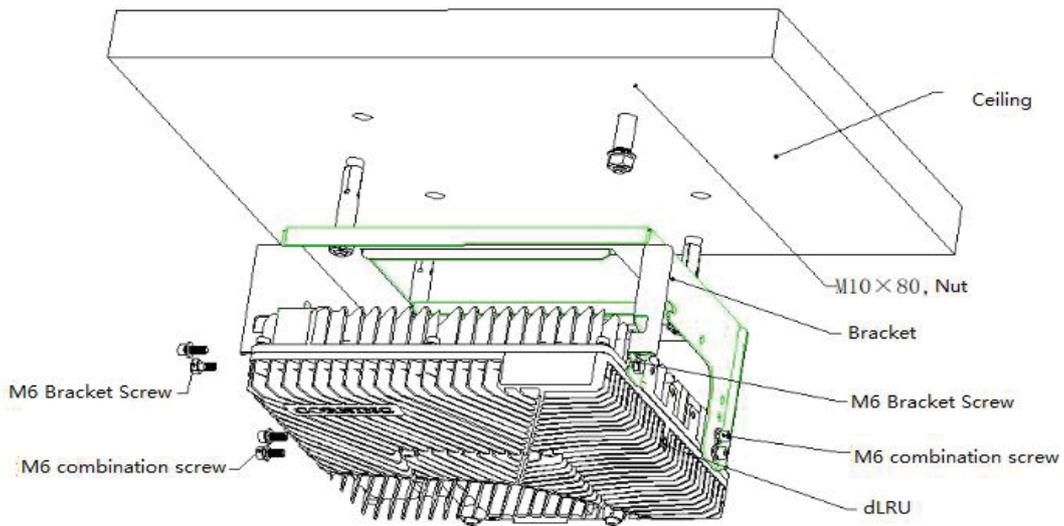
Figure 40. Single Unit Ceiling Installation
