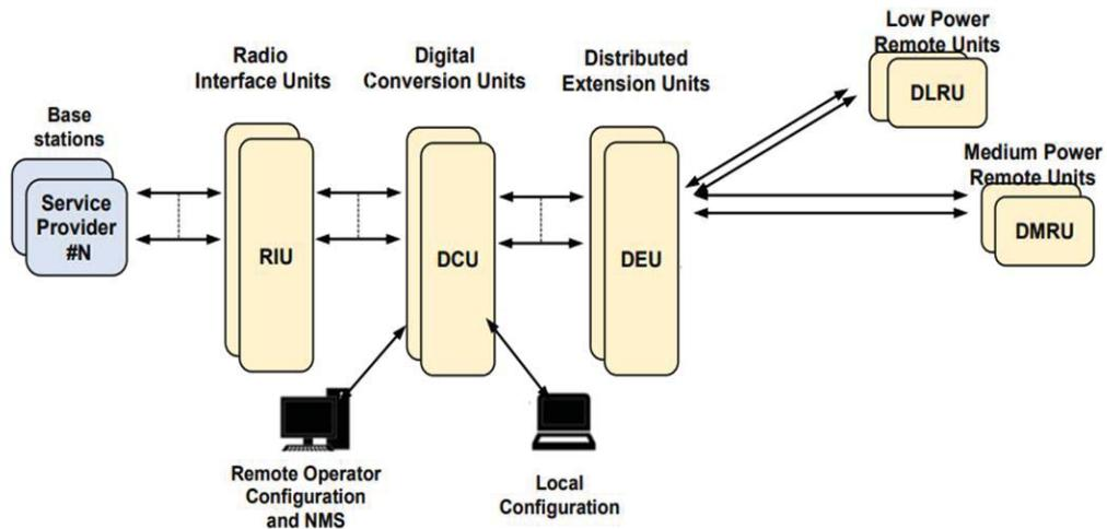
Figure 1. Architecture diagram
