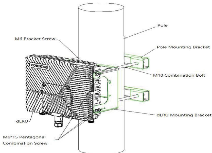
Figure 49. Diagram of Pole Installation for Single Unit
