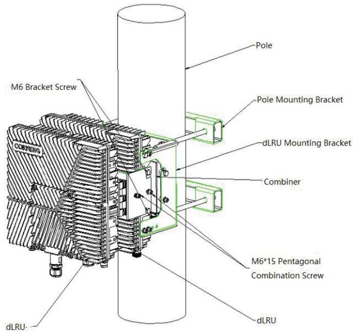
Figure 52. Dual Unit Installation Diagram
