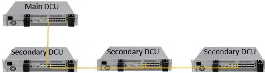
Figure 11. DCU Daisy Connection
