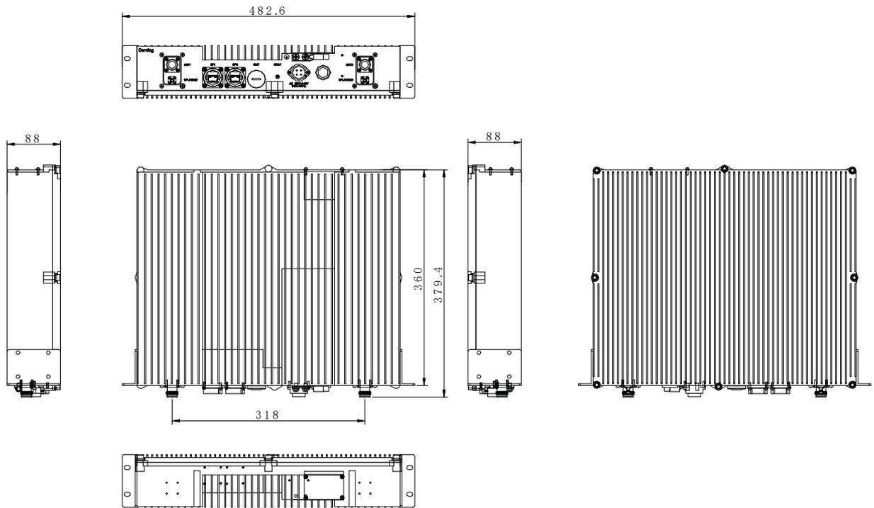
Figure 61. DMRU Dimensions - Without a Fan
