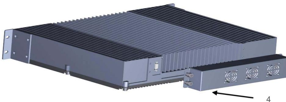
Figure 69. Fan Installation
