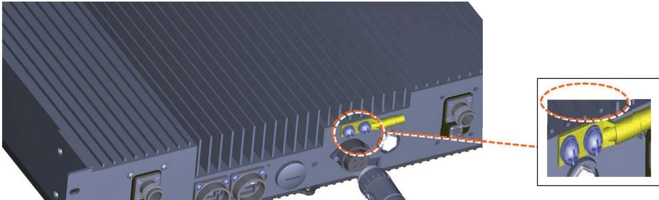
Figure 71. GND Connection
