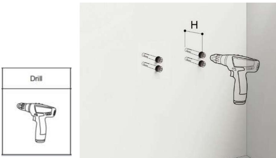
5. Attach the dowels, expansion screws or the like, and fasten the Bracket II to the wall.
