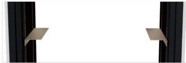
3. Place the EU in the rack and secure the EU using 2 screws M6×16 on both side and the Phillips screwdriver.
