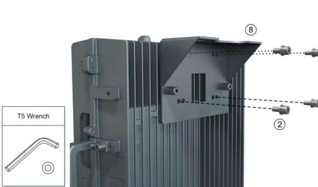
3. Mark the position of the drilling holes in the mounting Bracket II. Note:  $R = 13 \text{ mm}$ .
