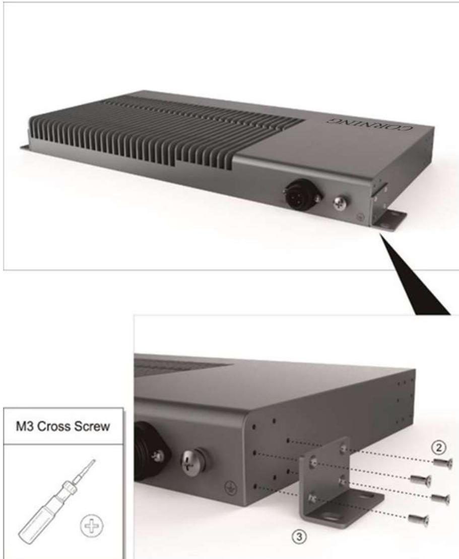
2. Mark 4 x  $\varnothing 6.8$  mm drilling holes sites for the hanger to be attached to the wall
