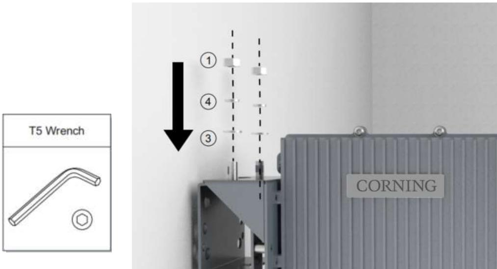
7. Fasten the Bracket I and II with screws M6×14.
