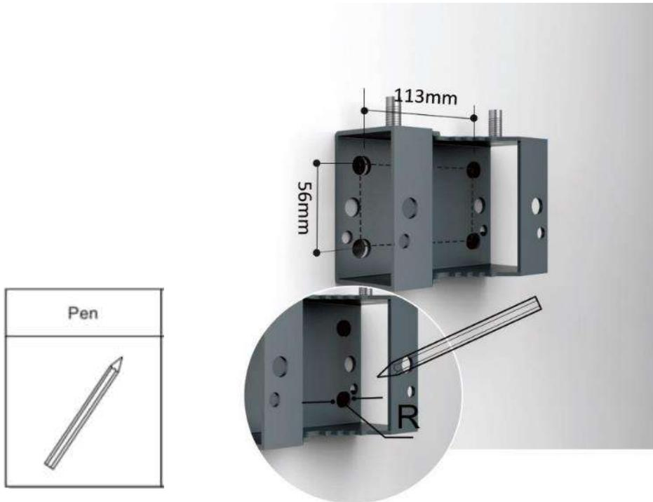
4. Drill 4 holes at the marked positions. Note:  $H = 70 \text{ mm}$
