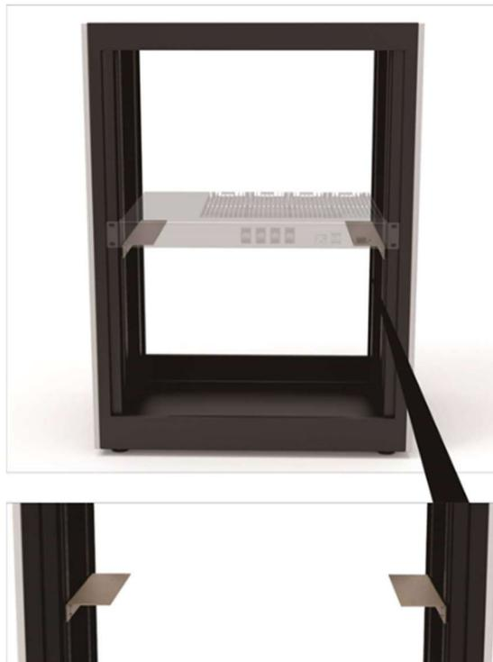
3. Place the AU in the rack and secure the AU using 2 screws M6×16 on both side and the Phillips screwdriver.
