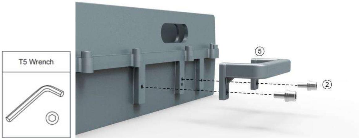
2. Attach and fasten the Bracket I to the back of M2RU with screws M6×14 using T5 Wrench.
