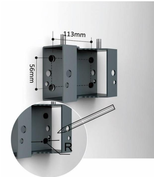
4. Drill 4 holes at the marked positions. Note:  $H = 70 \text{ mm}$
