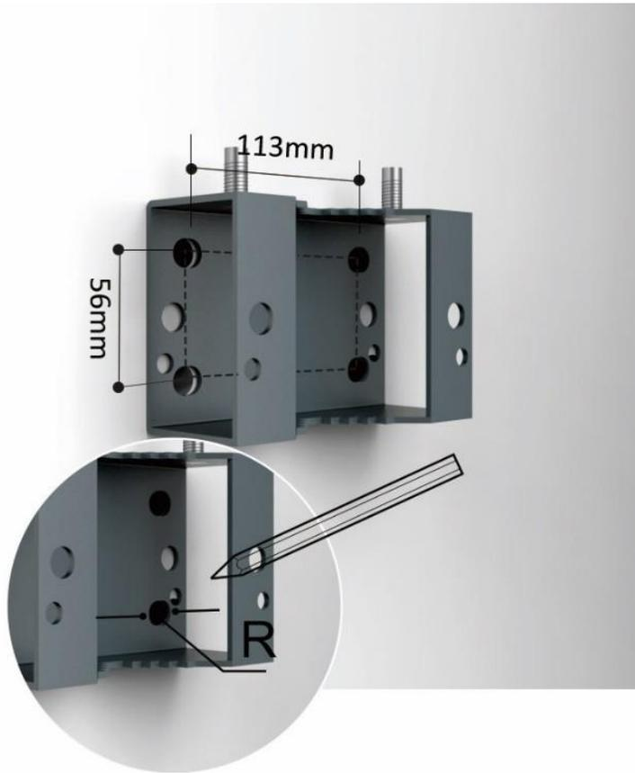
4. Drill 4 holes at the marked positions. Note:  $H = 70\text{ mm}$ .
