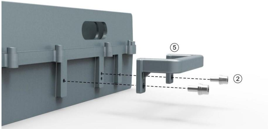
2. Attach and fasten the Bracket I to the back of M2RU with screws M6×14 using T5 Wrench.
