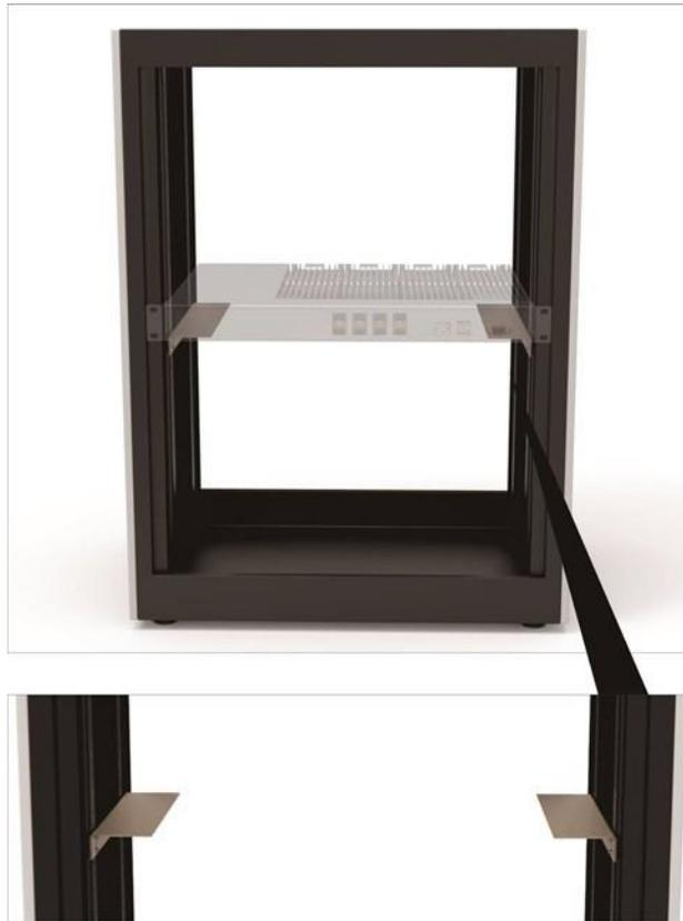
3. Place the AU in the rack and secure the AU using 2 screws M6x16 on both side and the Phillips screwdriver.
