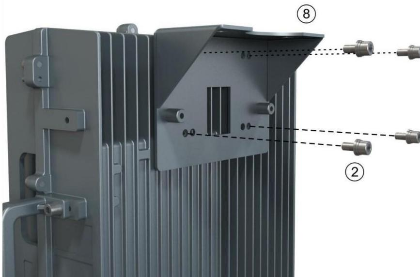
3. Mark the position of the drilling holes in the mounting Bracket II. Note:  $R = 13 \text{ mm}$ .
