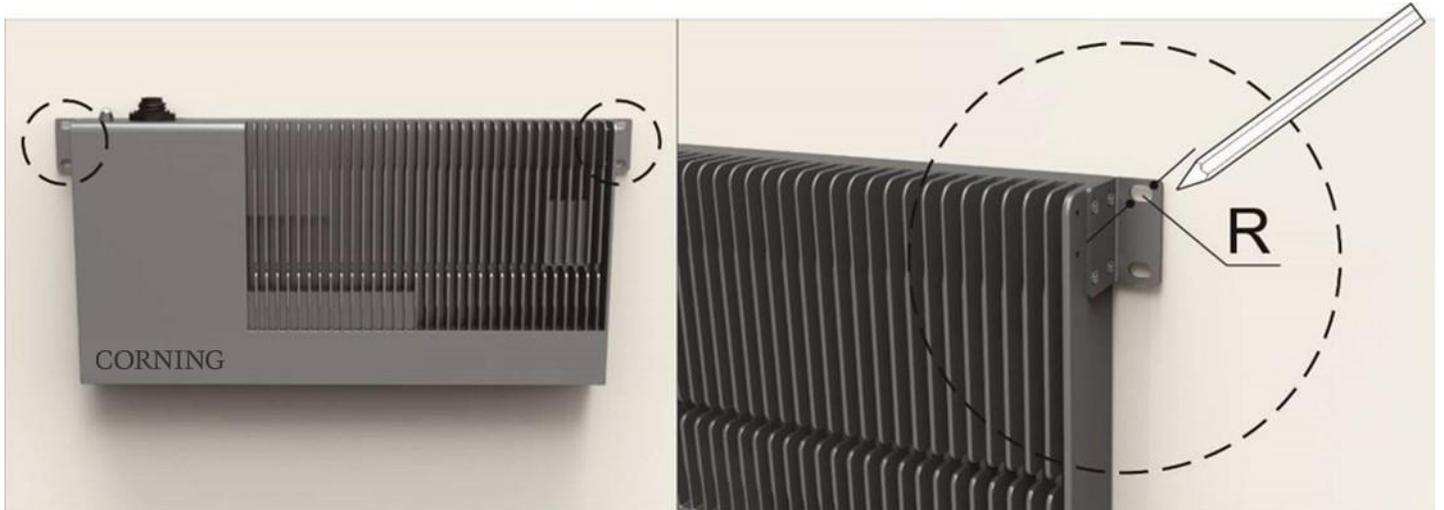
3. Drill 4 holes at the marked sites using percussion drill and embed 4x $\varnothing 10$  plastic expansion pipes. Note: H = 70mm. Fasten the case with 4xM6 expansion bolt.
