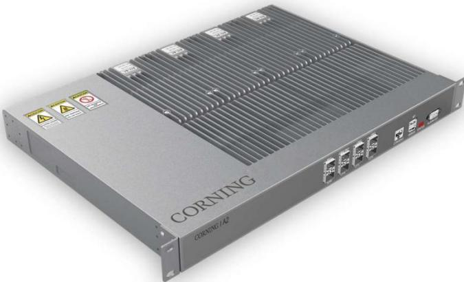
The E62-A2 – Access Unit Chassis is a standard 19-inch 1U rack-mounted shelf, which serves as the host for Everon™ 6200. The E62-A2 provides coupling access to radio signal sources of multioperator, multisystem, and multiband, forming digital optical signals and distributing static capacity distribution to fiber-connected slave devices. One A2 supports up to eight optical interfaces connected to EUs (Expansion Units) or RUs (Radio Units).
