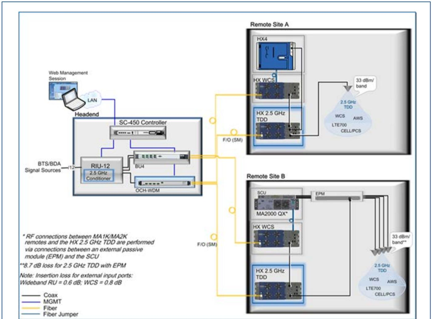
HX 2.5 GHz TDD – SISO Architecture with an existing HX4 and MA2000 QX, Sharing a Common Headend | Figure 1-2
