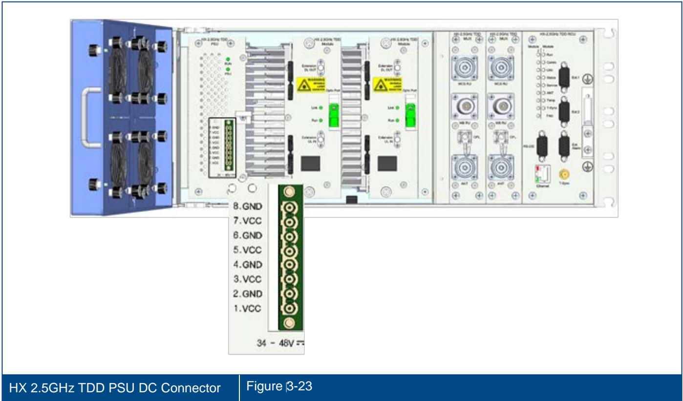
HX 2.5GHz TDD PSU DC Connector | Figure 3-23
