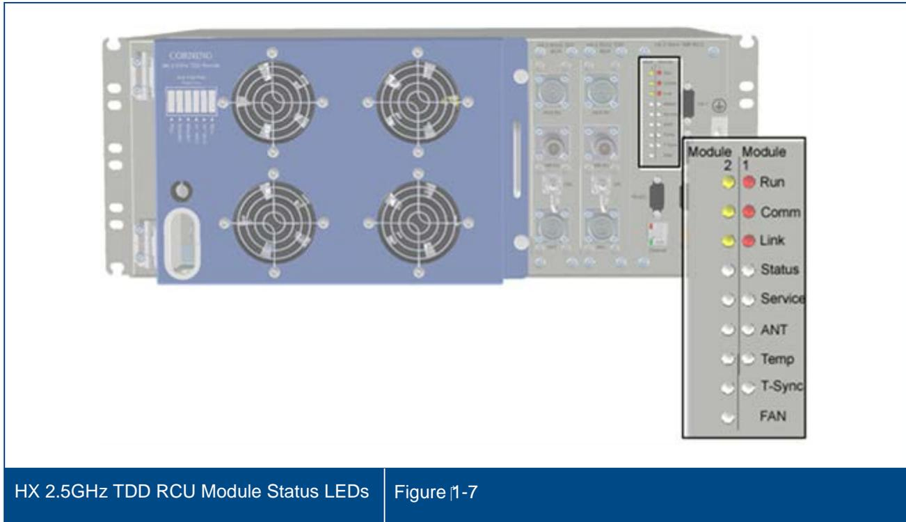
Note: Module 1 and Module 2 LEDs correspond to installed modules [Module 1 for ANT. 1 (SISO); Module 2 for ANT. 2 (MIMO)].
