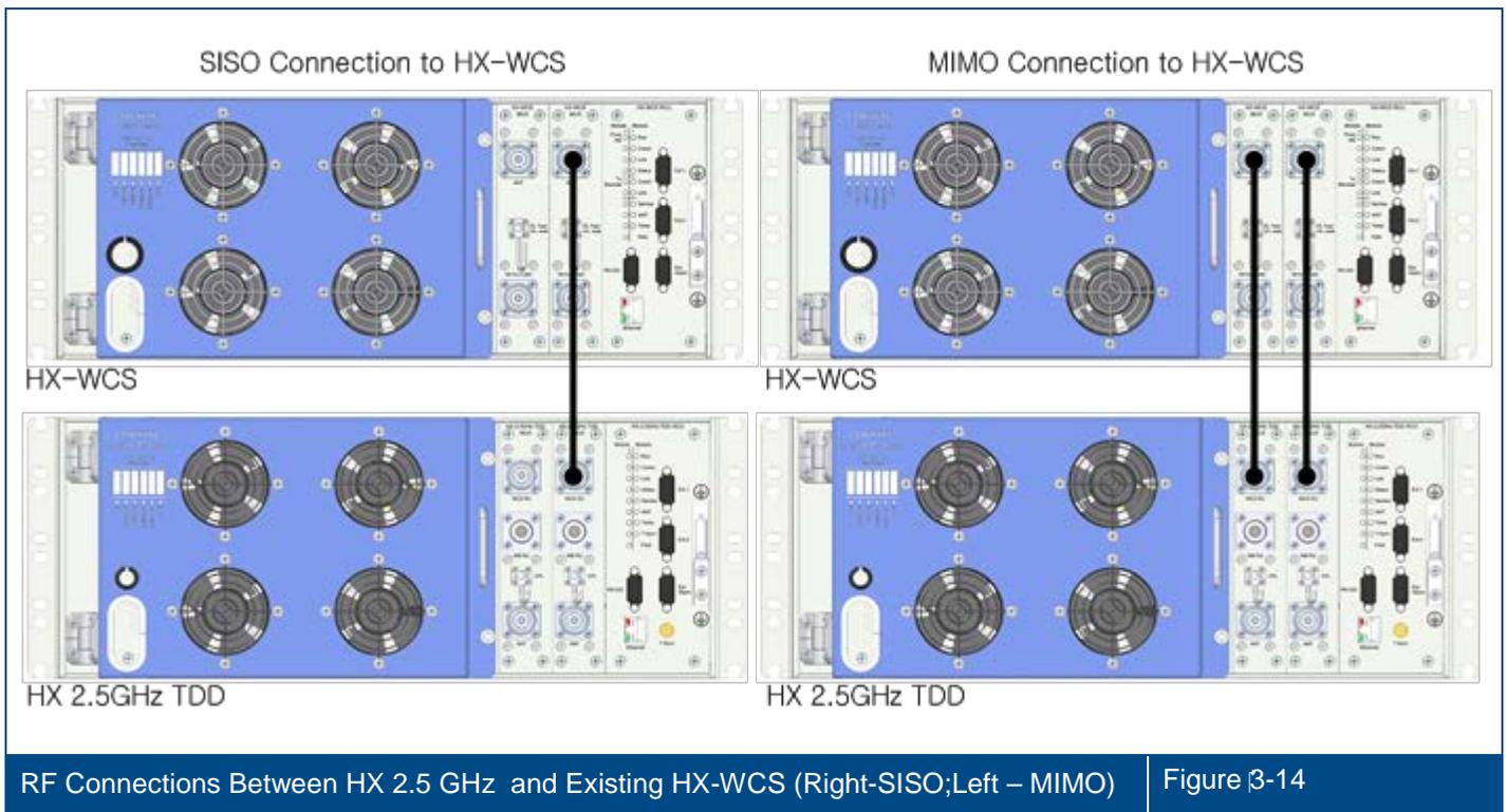
2. Connect broadband antenna coax to HX-2.5 GHz TDD MUX module “ANT” port of (two for MIMO models) and to broadband DAS antennas.
