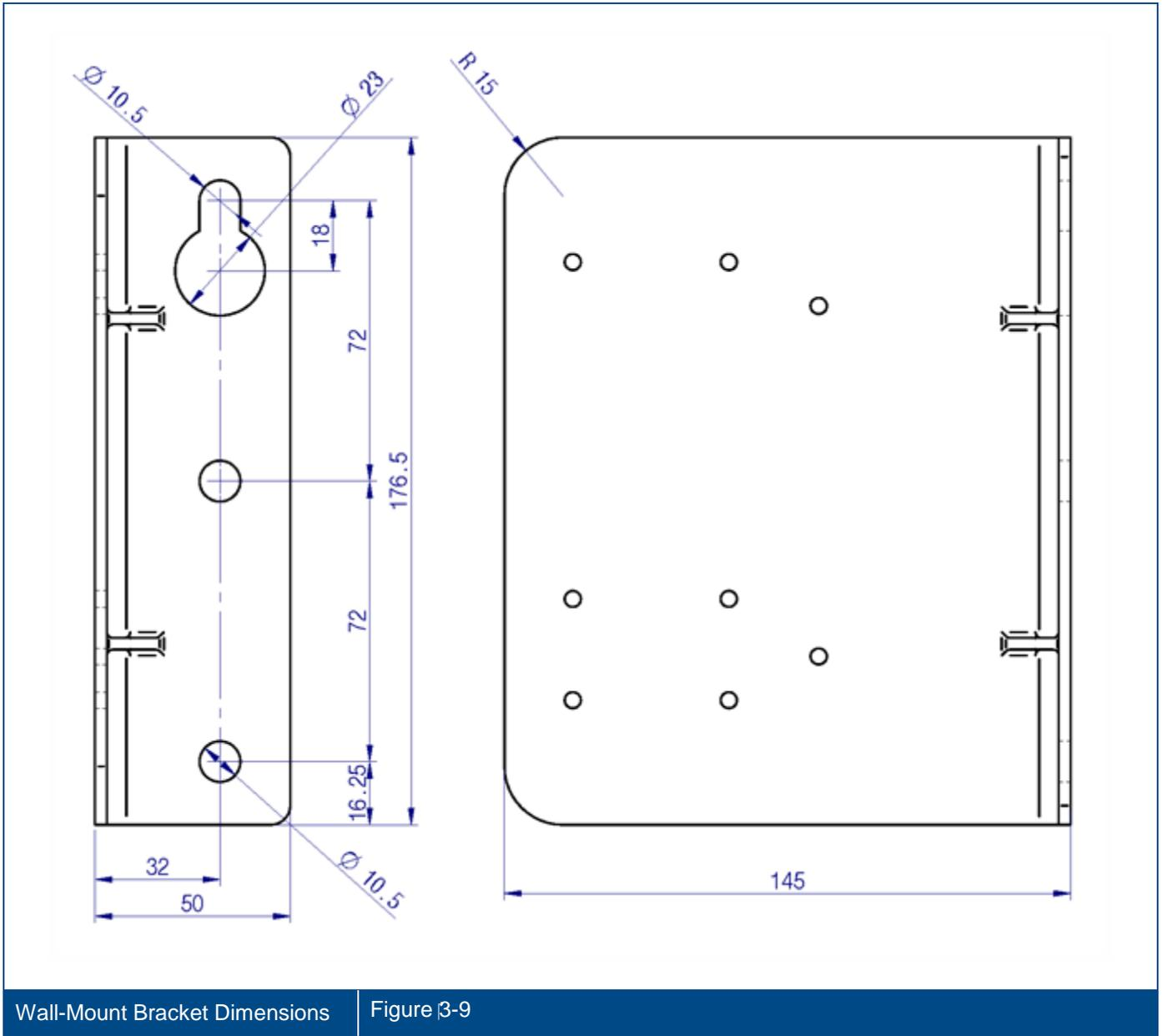
4. Using bracket holes as a template, mark holes for drilling in wall.
