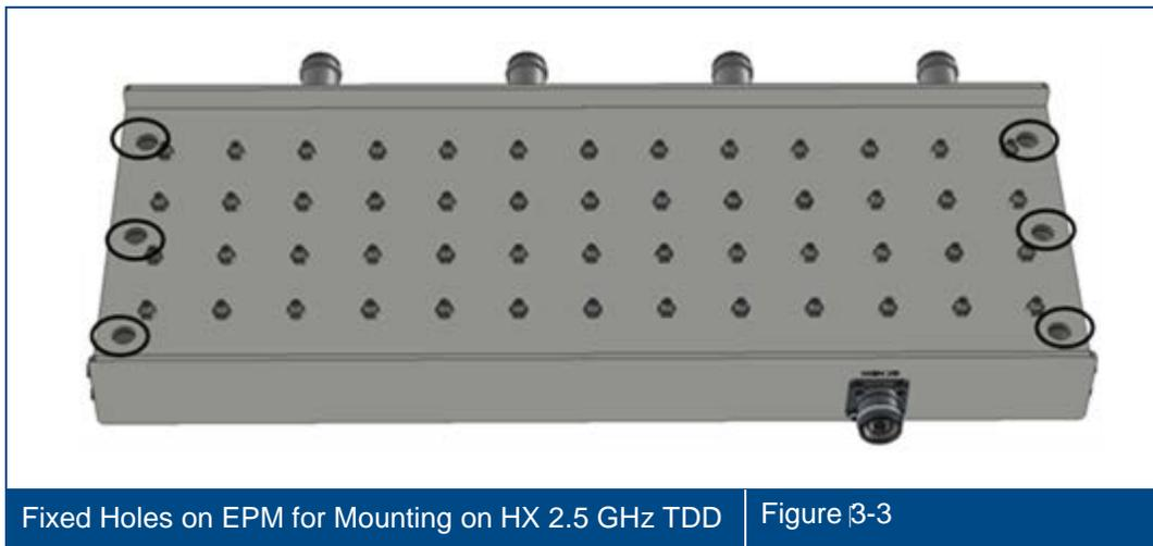
3. Place the EPM onto the top of the HX 2.5 GHz TDD unit and using six UNC 6-32, 11 mm screws (not provided), assemble the EPM onto the HX 2.5 GHz TDD unit. See Figure 3-4.
