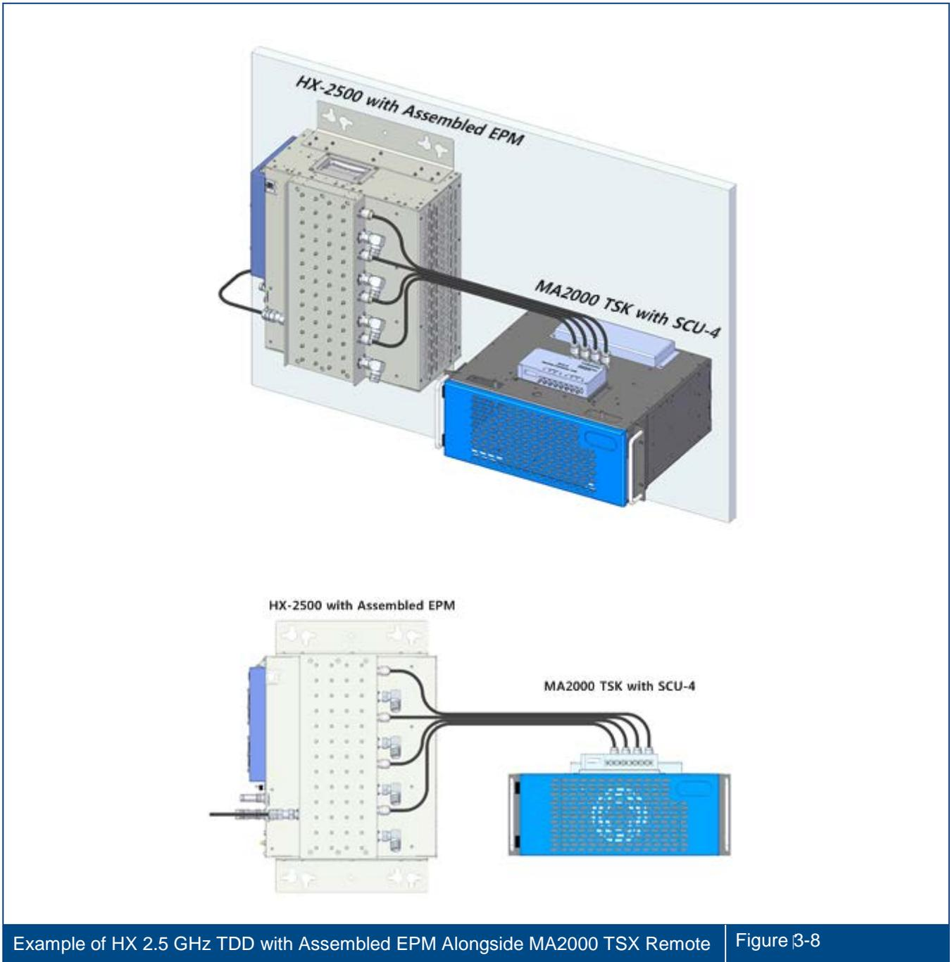
Example of HX 2.5 GHz TDD with Assembled EPM Alongside MA2000 TSX Remote | Figure 3-8
