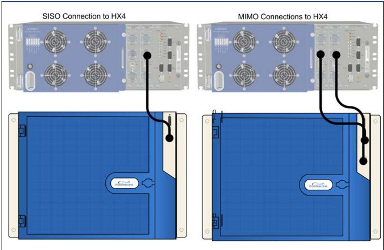
2. Connect broadband antenna coax to the HX-2.5 GHz TDD MUX module “ANT” port (two for MIMO models) and to broadband DAS antennas. Refer to Figure 3-13 for example.
