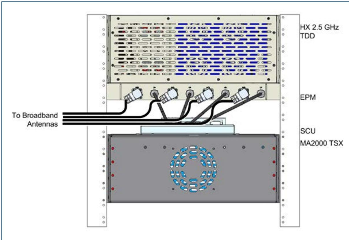
Example of Connections between EPM and MA2000 TSX | Figure 3-17
