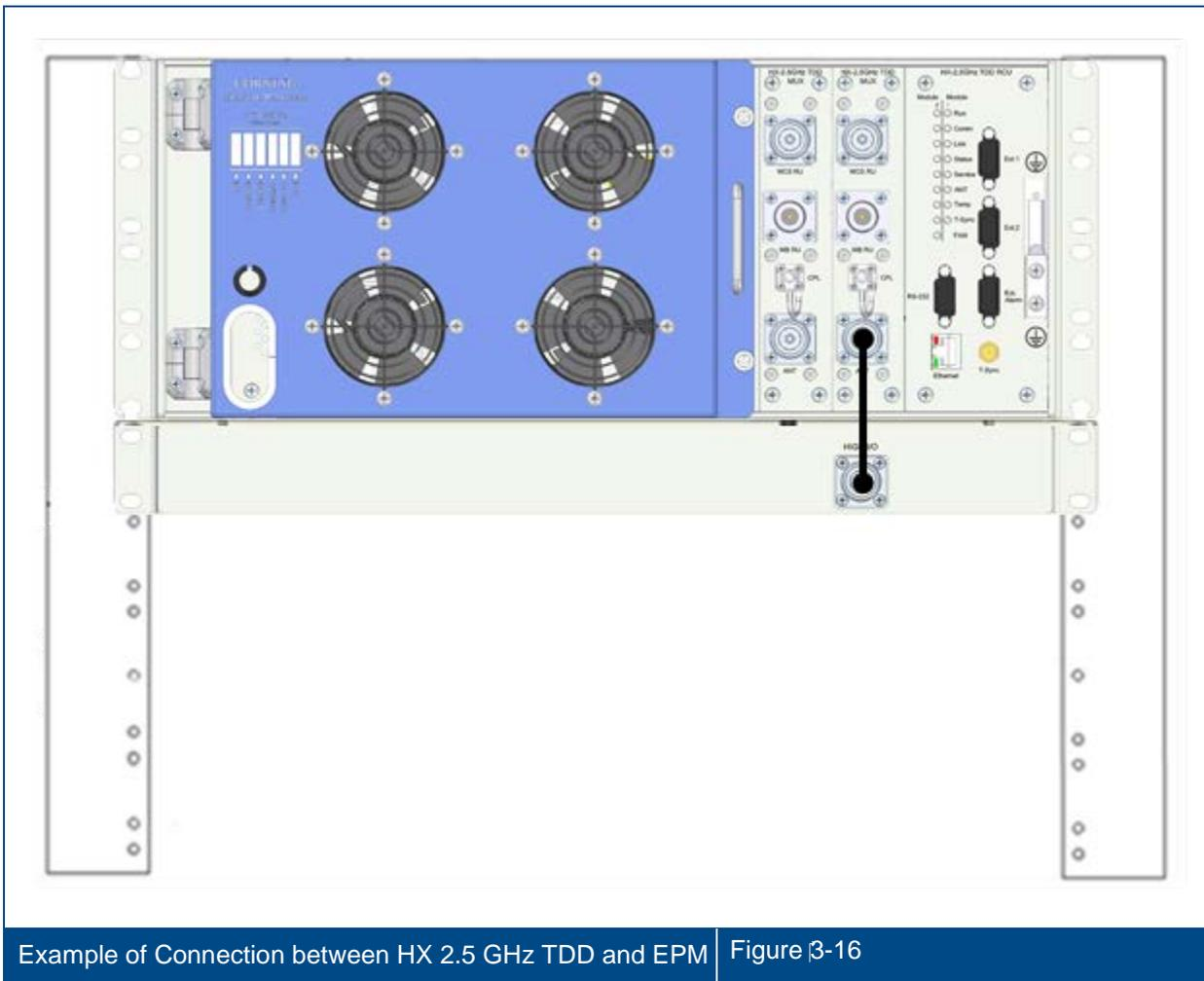
2. Connect the four rear panel EPM low-band N-Type input ports to the corresponding SCU N-Type ANTENNA PORTS”.
