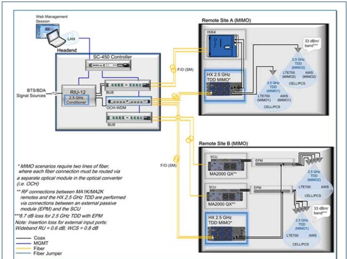
HX 2.5 GHz TDD – MIMO Architecture with an existing HX4 and MA2000 QX, Sharing a Common Headend | Figure 1-3
