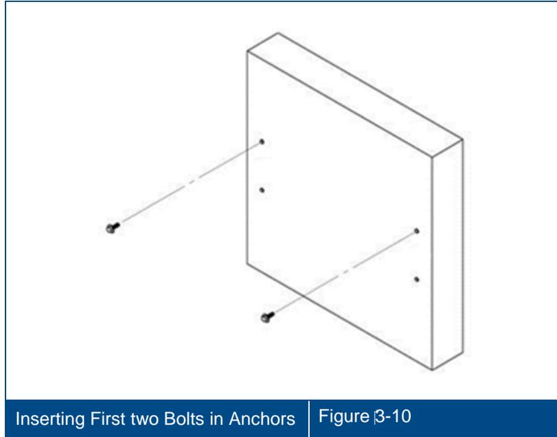
6. Hang the unit and bracket assembly onto the two bolts using the key holes.
