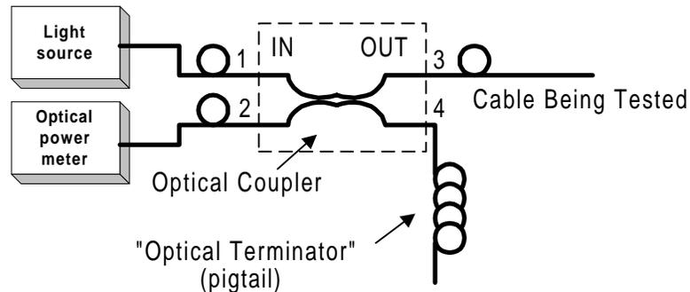
**Figure 20 – Optical Return Loss Measurement**
