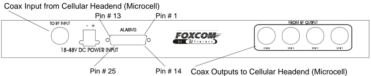
**Figure 3 - Base Unit Back Panels 4 ports**
