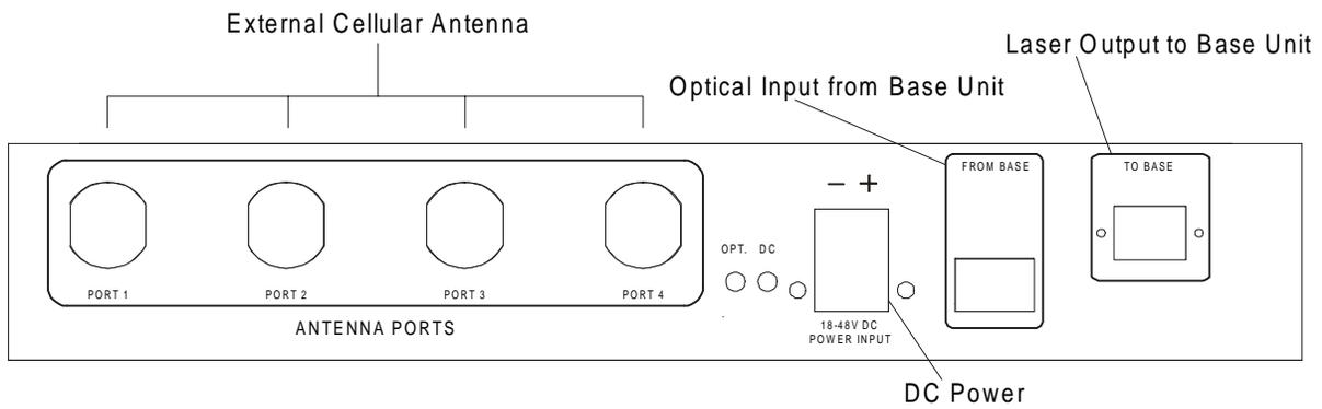
**Figure 8 - Remote Hub Unit Front Panel**
