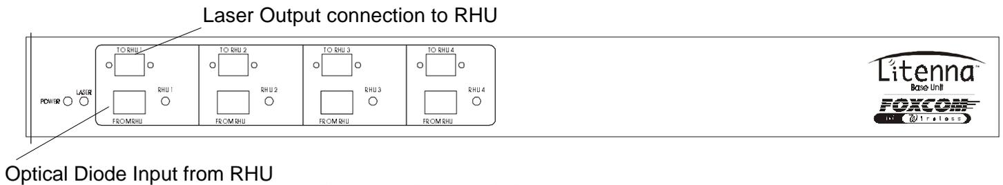
**Figure 2 - Base Unit Front Panel 4 ports**
