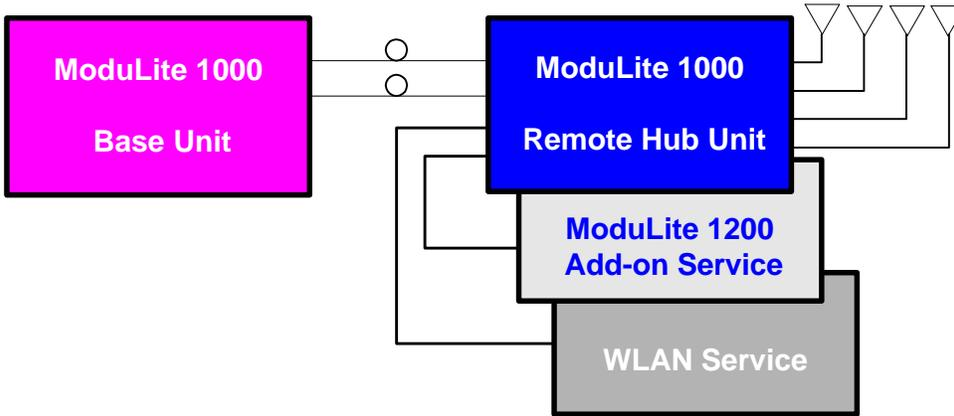
**Figure 5: MobileAccess 1000/1200 BU – RHU Plus Add-on Plus WLAN Configuration**
