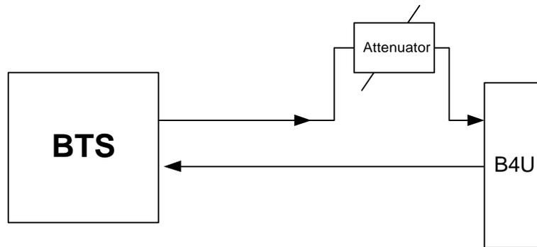
Figure 3-6: Example: Two port BTS/RBS connected to B4U.
