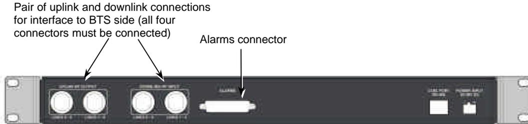
Figure 2-5. Base Hub Unit Rear Panel (RF Connections)
