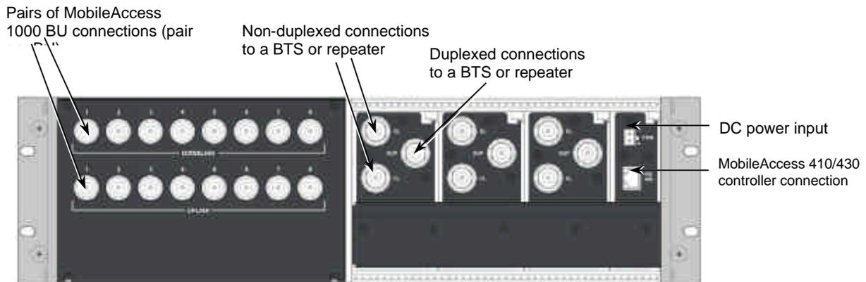
Figure 2-2. RIU Rear Panel showing the RF Connection
