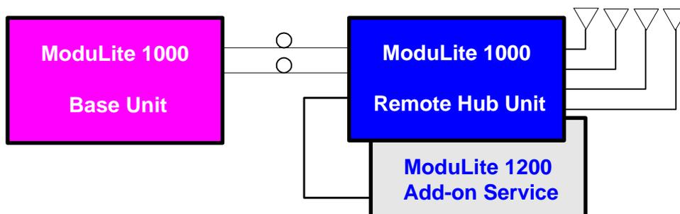
**Figure 4: MobileAccess 1000/1200 BU – RHU Plus Add-On**
