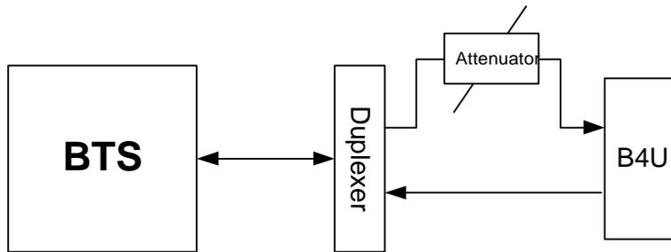
**Figure 3-4: Example: One port BTS/RBS connected to 1BFU**
