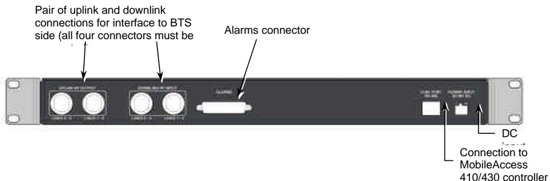
Figure 3-3. Base Hub Unit Rear Panel (RF Connections)
