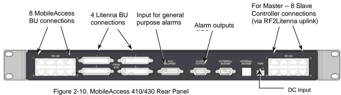
Figure 2-10. MobileAccess 410/430 Rear Panel
