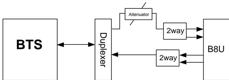
**Figure 3-5: Example: One port BTS/RBS connected to 1 B8U .**
