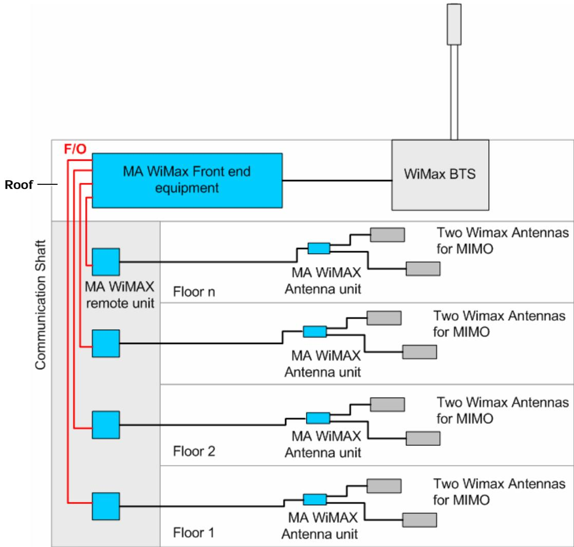
Figure 1. MA WiMAX System Architecture
