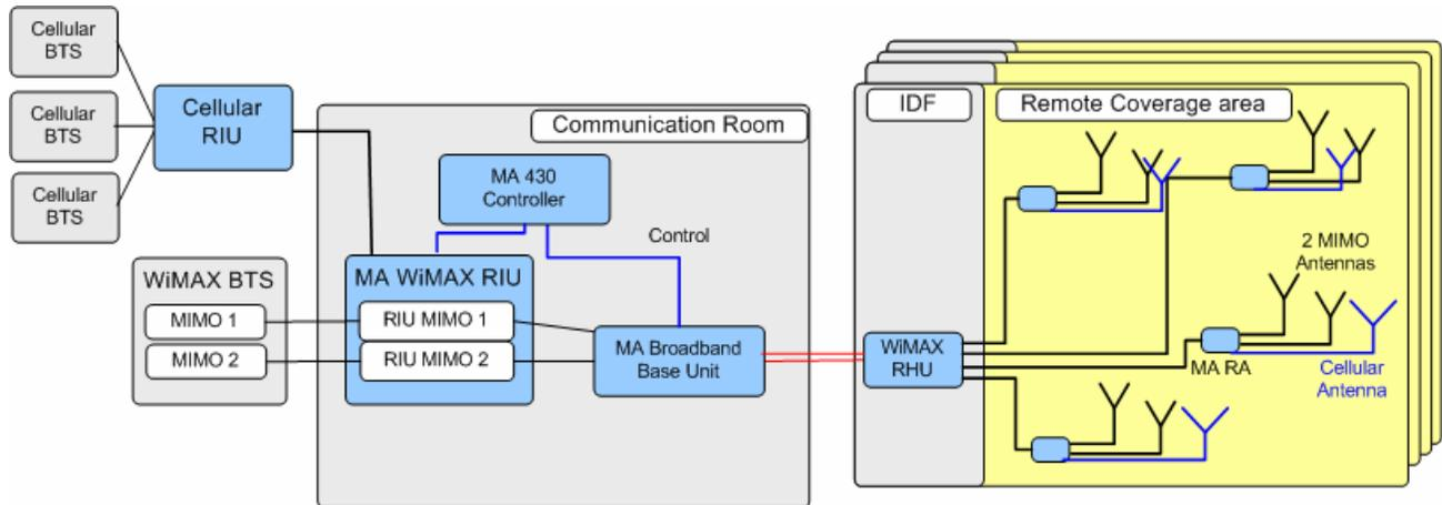
Figure 1-4. Architecture of a converged Cellular-WiMAX system
