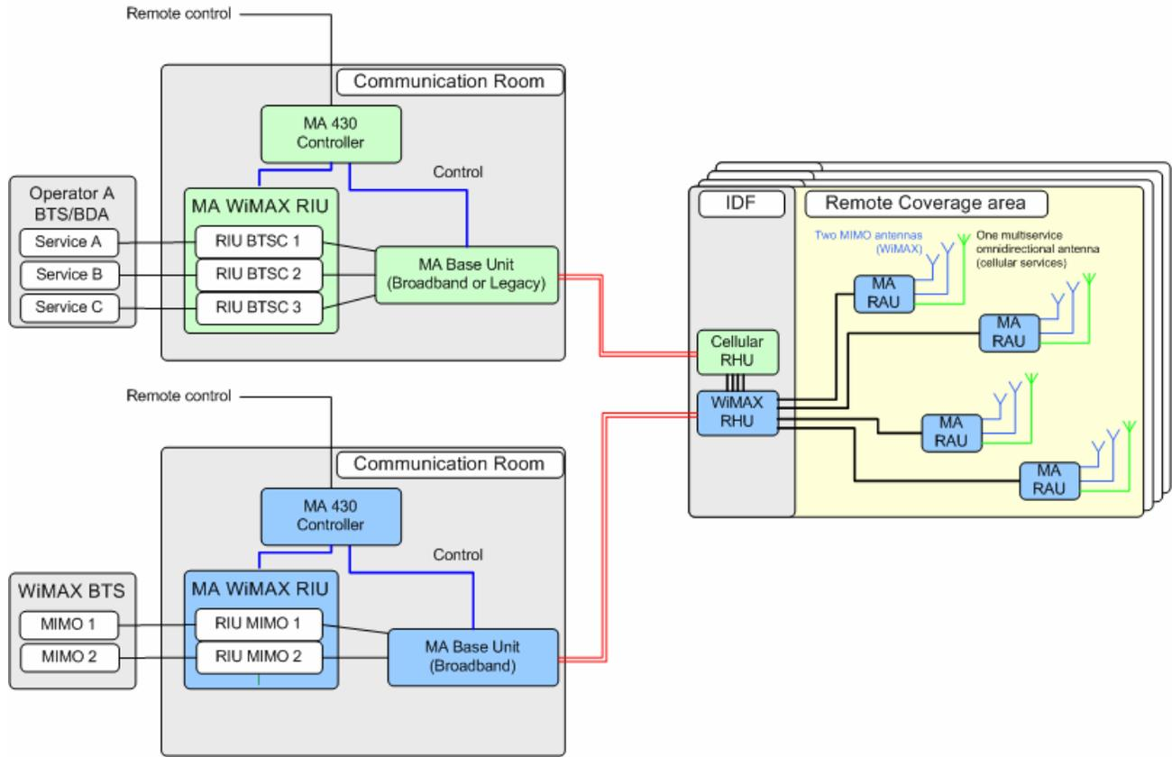
Figure-1-3 –Architecture of MA WiMAX System Converged with MA 1000 System Services
