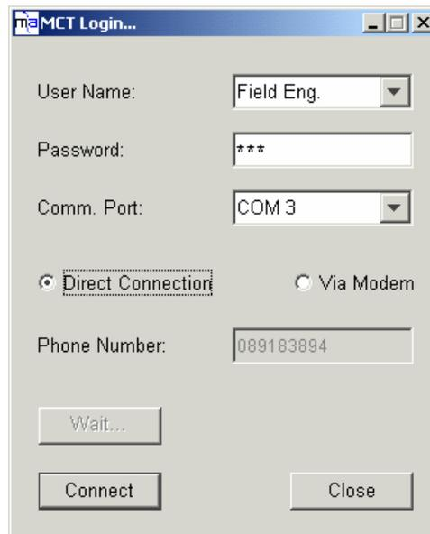
3. To access the MCT screen at a level that provides access to configuration options, select the **User Name 'Field Eng'** and enter the default Engineering password **'eng'**.
