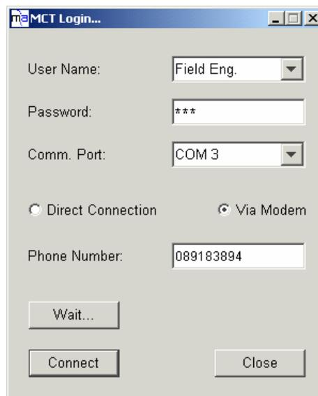
3. To access the MCT screen at a level that provides access to configuration options, select the **User Name 'Engineering'** and enter the default Engineering password **'eng'**
