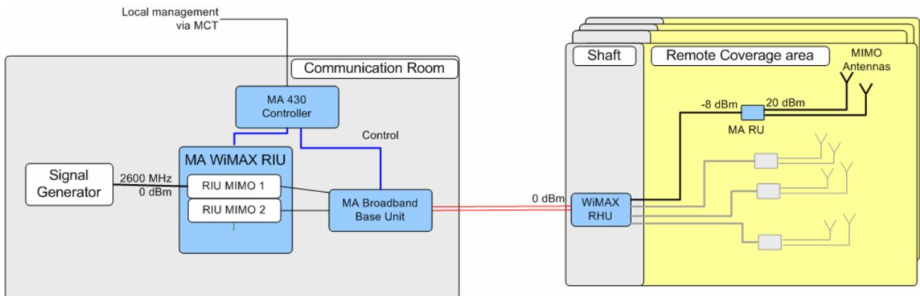
The adjustment procedure can be performed simultaneously for all RHUs and Remote Antennas in the system from the configuration dialog of *any of the RIUs* in your WiMAX system.
