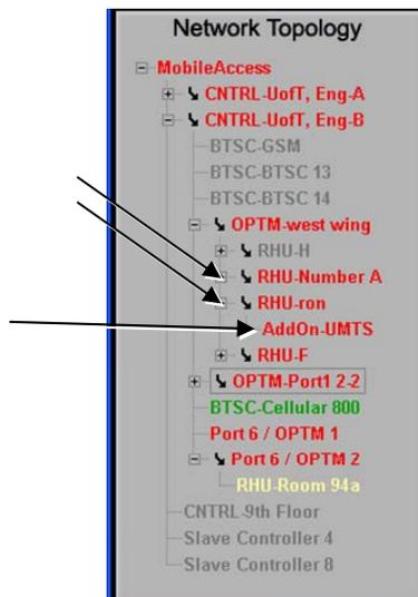
**IMPORTANT NOTE!** If the RHUs are not all visible, reset or power cycle the Base Units to which it is connected. If this does not resolve the problem, troubleshoot the optical links for dirt or other problems.
