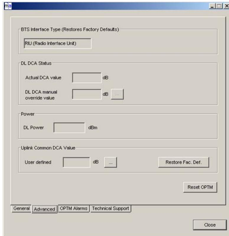
4. The DL gain may be set automatically (AGC) or manually (DCA). To control the **DL gain control**, set the **DL AGC Mode** in the **Advanced** tab:
