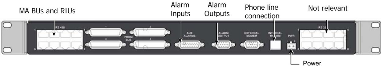
Figure 2-7. MobileAccess Controller Rear Panel
