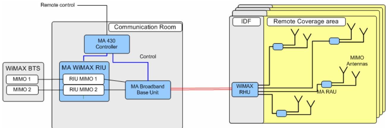
Figure 1-2. Architecture of a basic MA WiMAX system
