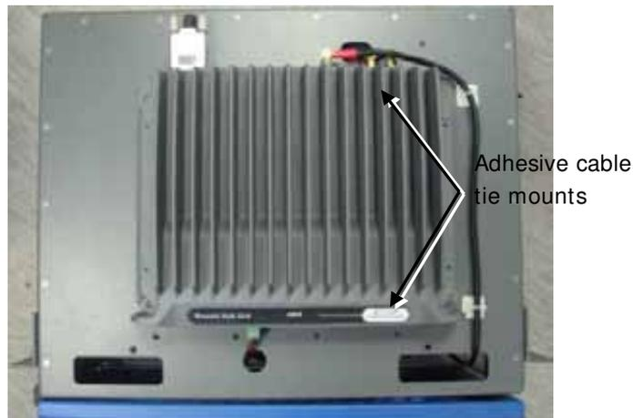
Figure 4-11. Secured High-Band connection
