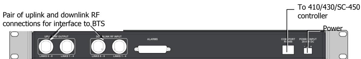
Figure 11. BU Rear Panel (RF Connections)
