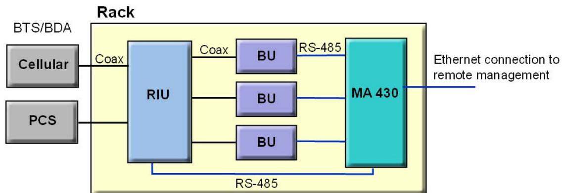
Figure 14. Example of Single-building Topology Communication Room Installation
