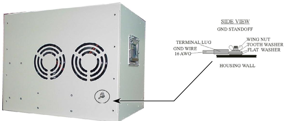
**Figure 3-6: Grounding Located at the Rear of the Unit**
