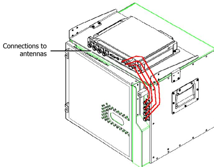
**Figure 3-12. Illustration of RC Antenna port connections**
