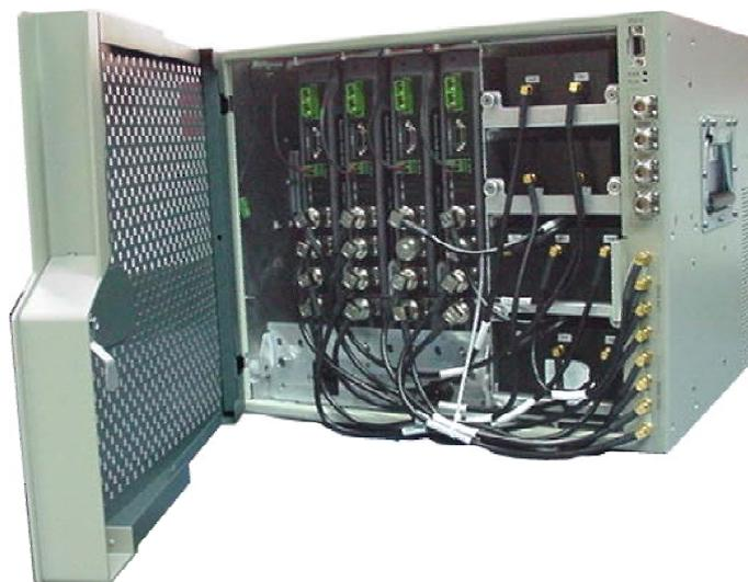
**Figure 4-3. RC Open Cabinet with Internal Cabling**
