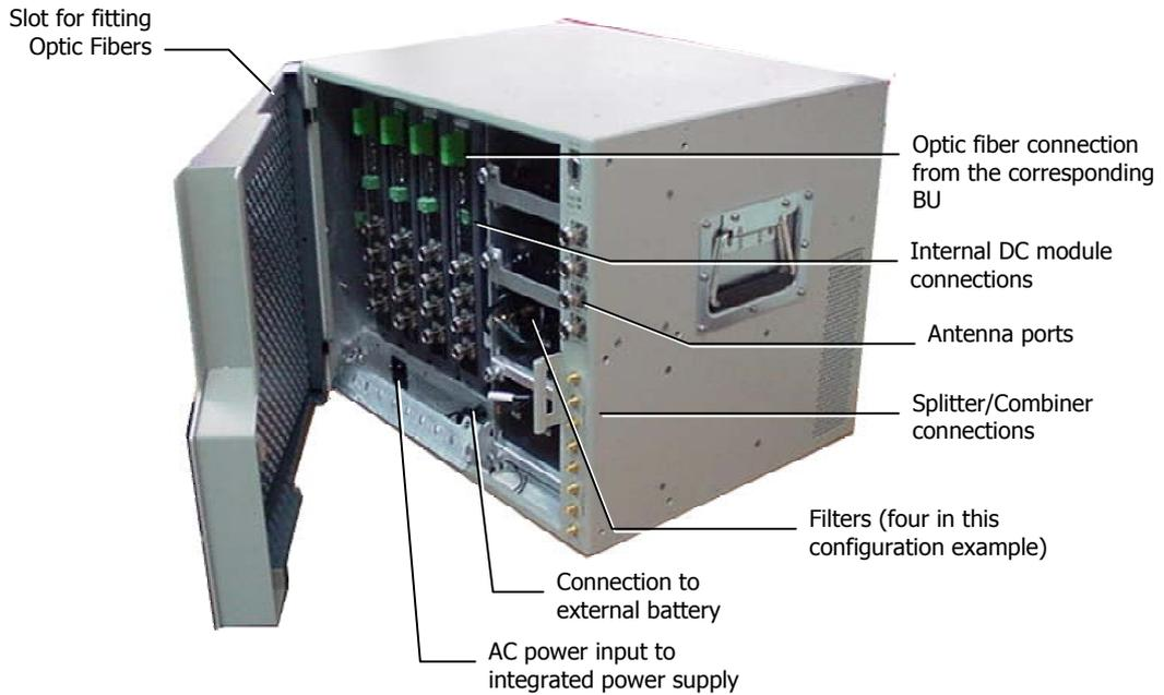
**Figure 4-2. RC 2000 Open Cabinet View (without internal connections)**
