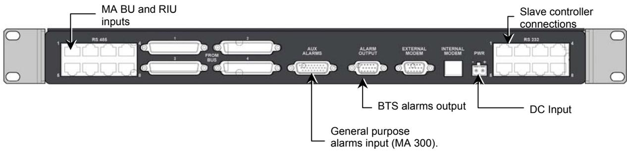
**Figure 4-20. MobileAccess 410/430 Rear Panel**
