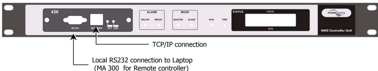
Figure 4-19. MobileAccess 430 Front Panel
