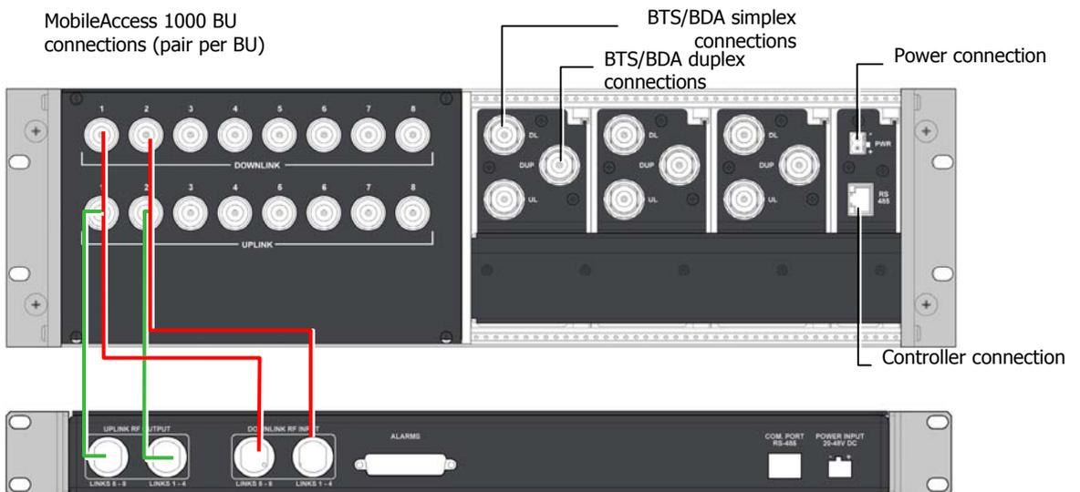
**Figure 4-14. RIU Rear Panel showing the RF Connection**
