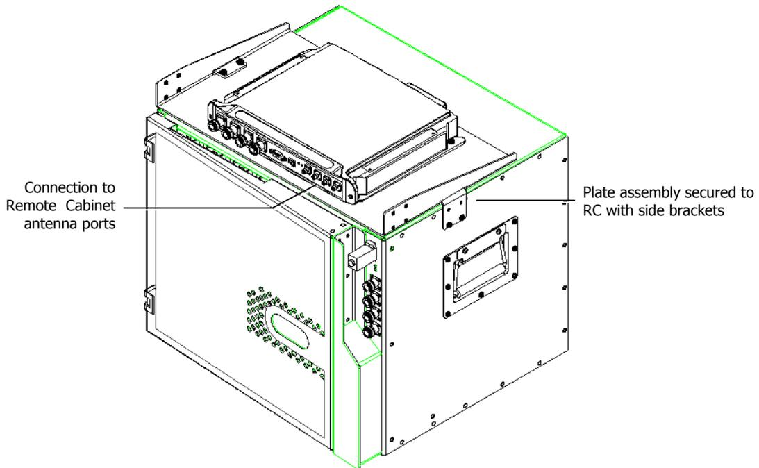
**Figure 3-11. Illustration of MA 850 Mounted on MA 2000 RC**
