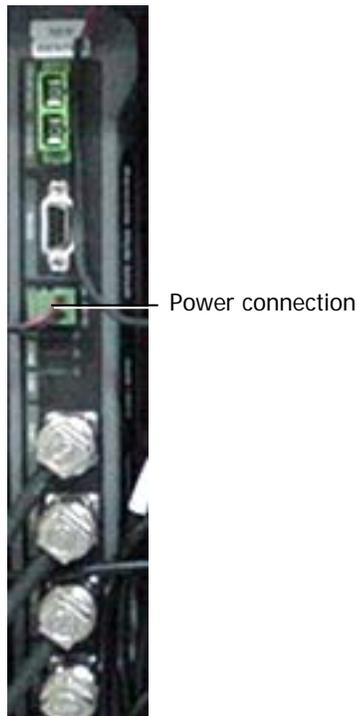
*Figure 4-10. RHU 2000 Fiber Optic and internal power connections*
