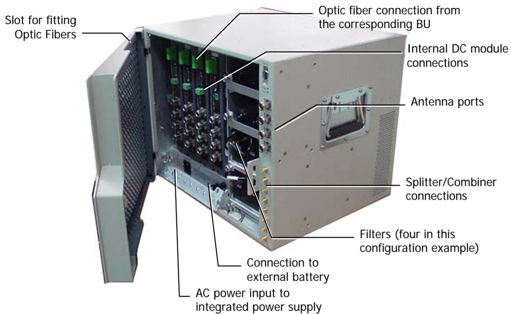
Figure 2-2. RC 2000 Open Cabinet View (without internal connections)
