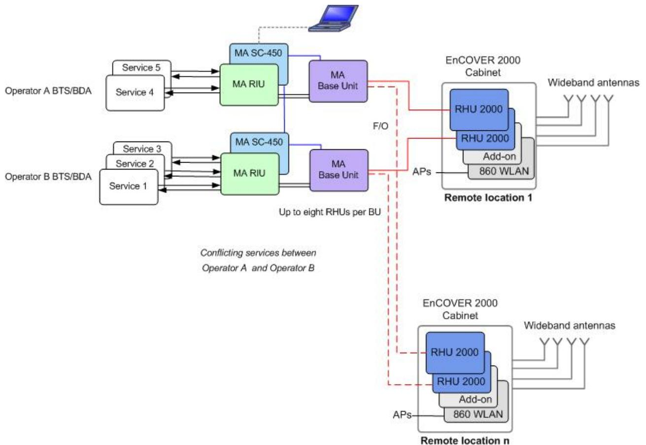
Figure 1-3. Example of MA 2000 Cabinet Architecture
