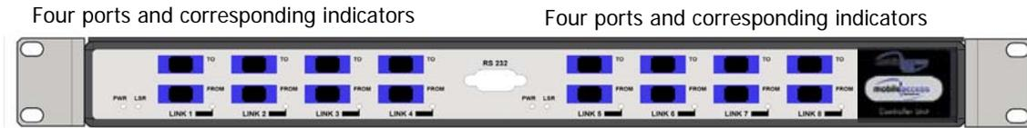
Figure 2-15. Eight-Port MA BU Front Panel
