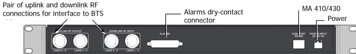
Figure 2-17. MA BU Rear Panel (RF Connections)
