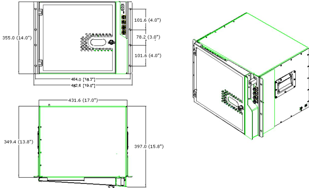
Figure 4-8. MA 2000 Cabinet Rack Mount Assembly
