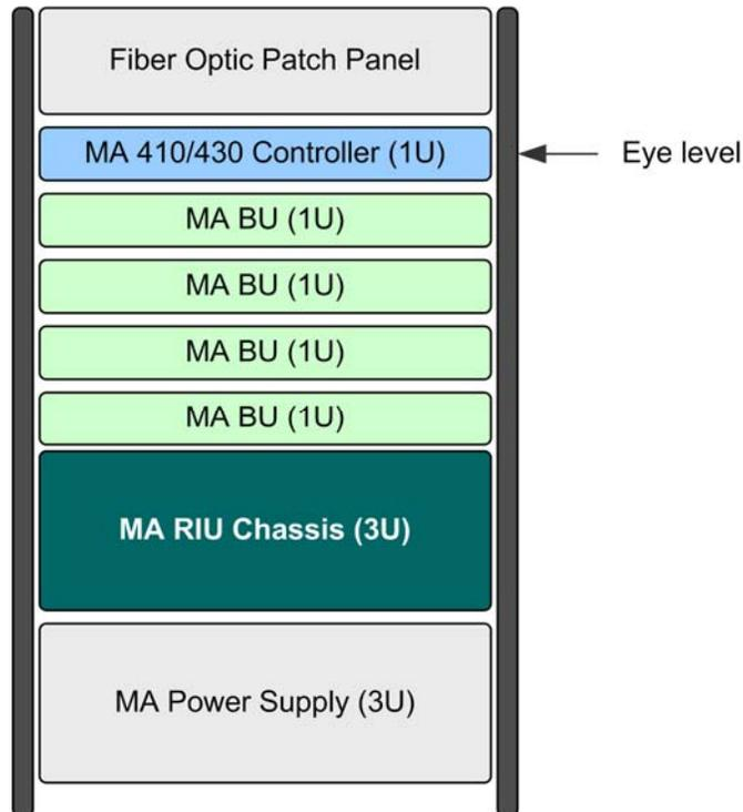
Figure 4-1: Recommended Order in the Communication Room Rack
