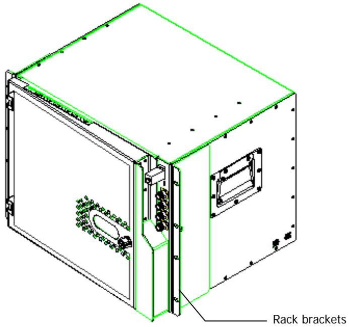
Figure 4-9 . MA 2000 RC Rack Model
