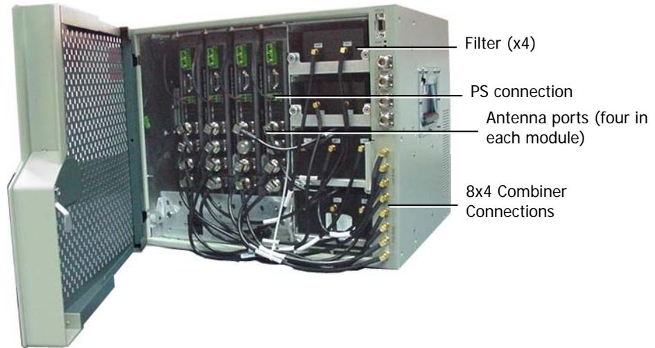
Figure 2-3. RC Open Cabinet with Internal Cabling
