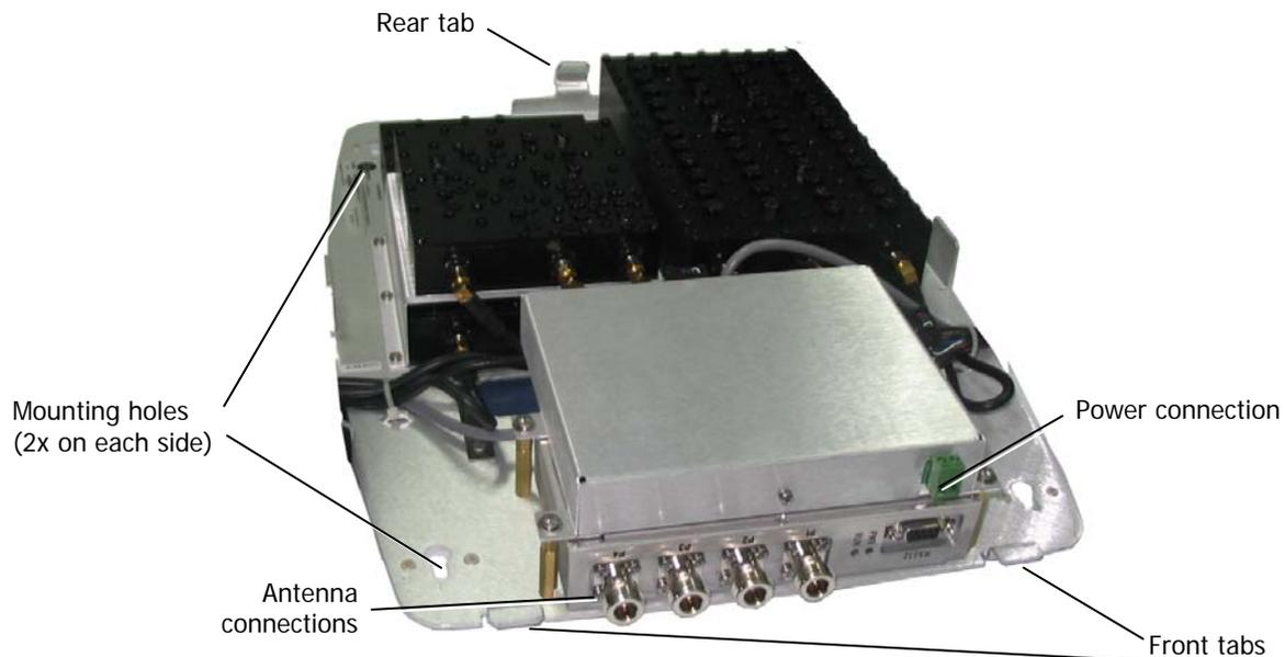
Figure 4-14. MA 2000 Lite Prepared for Mounting
