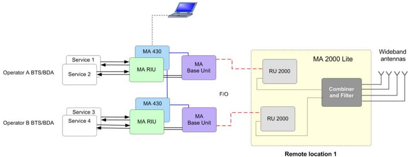
Figure 1-4. Example of MA 2000 Lite Architecture
