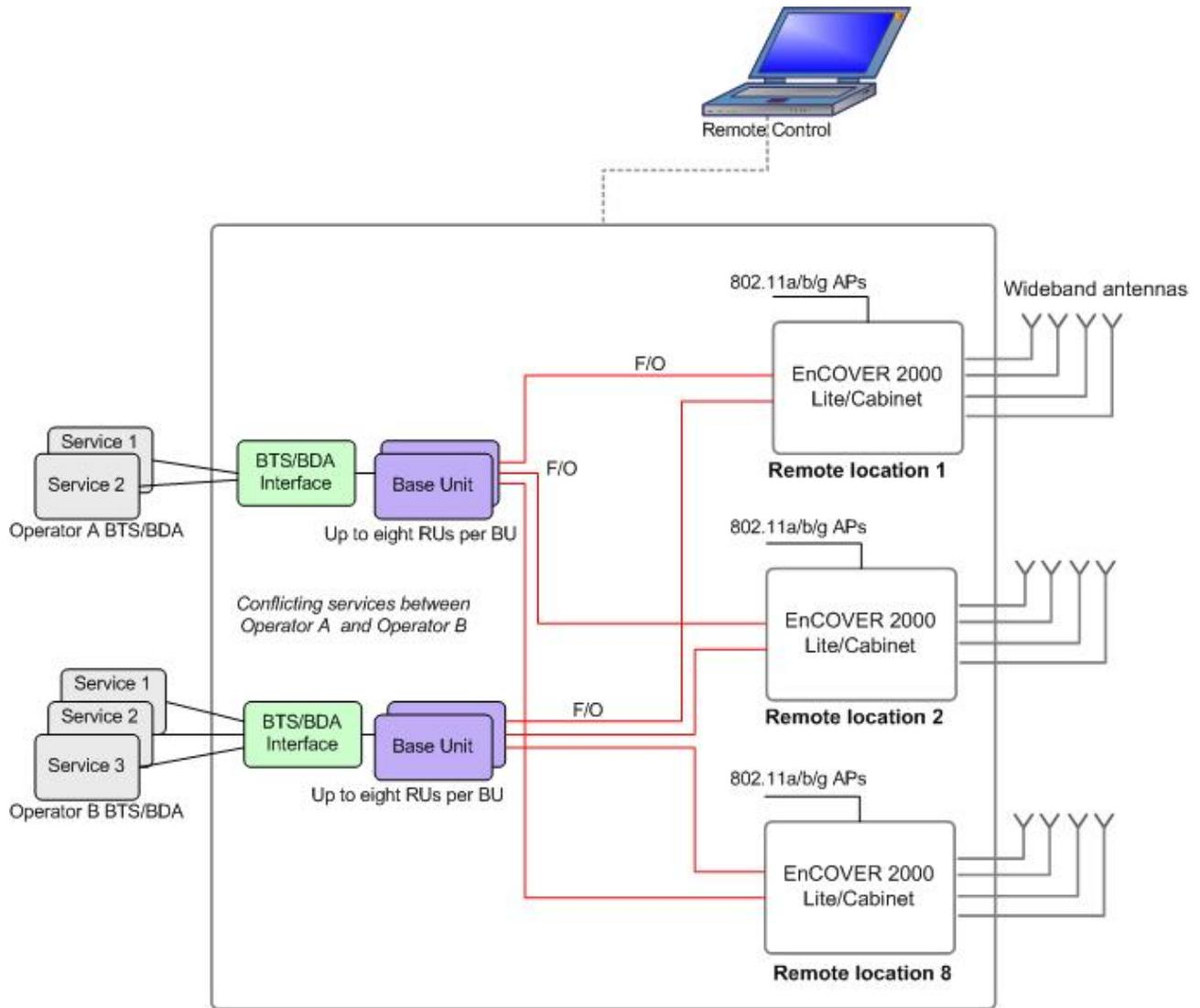
Figure 1-2. System Architecture
