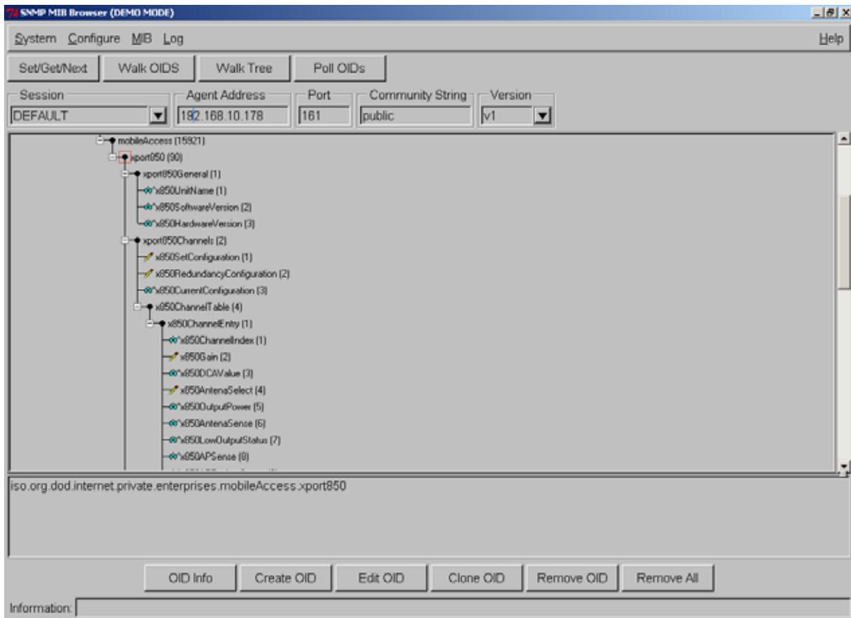
Figure 5-1. MIB Tree with Loaded MobileAccess 850 Files
