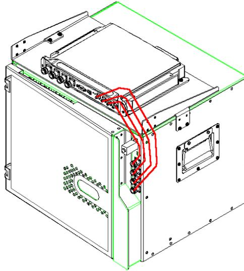
*Figure 3-7. Illustration of RC Antenna port connections*
