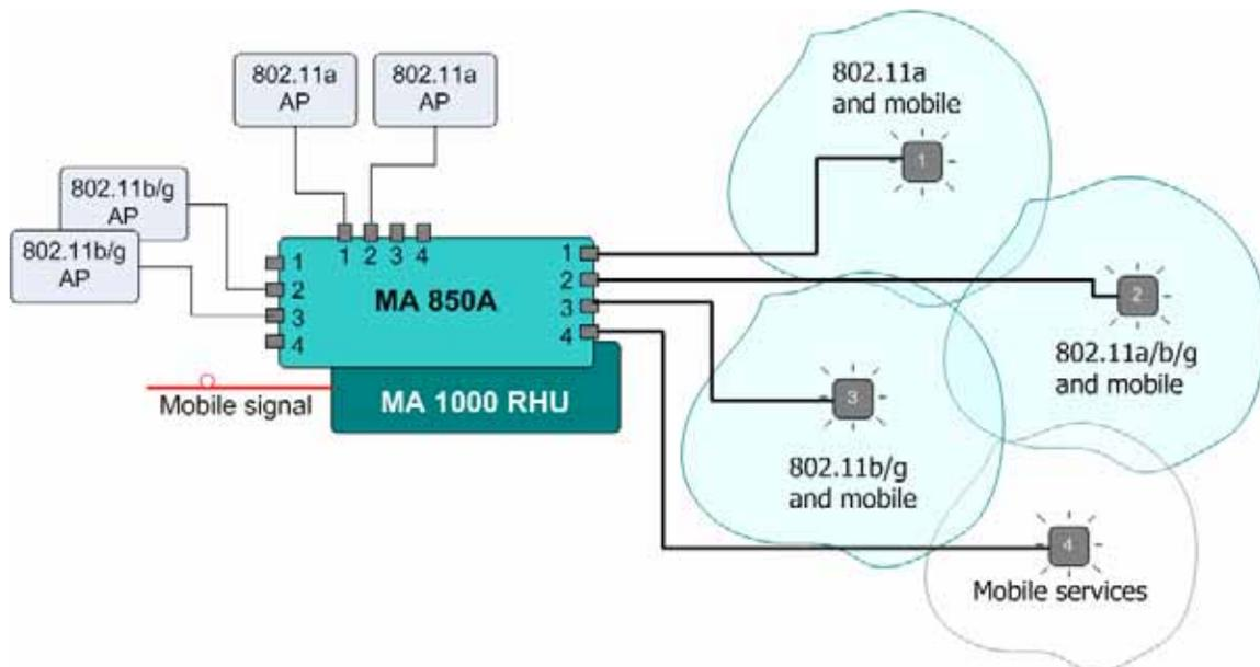
Figure 1-9. Example of 802.11a/b/g and Mobile Signal Distribution
