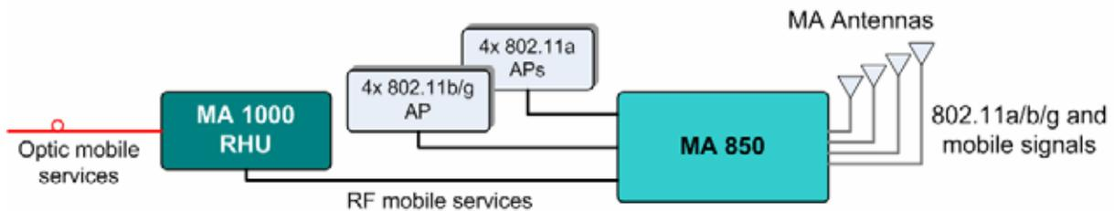
Figure 1-4 MA 850A1 as Add-On to MA 1000 System
