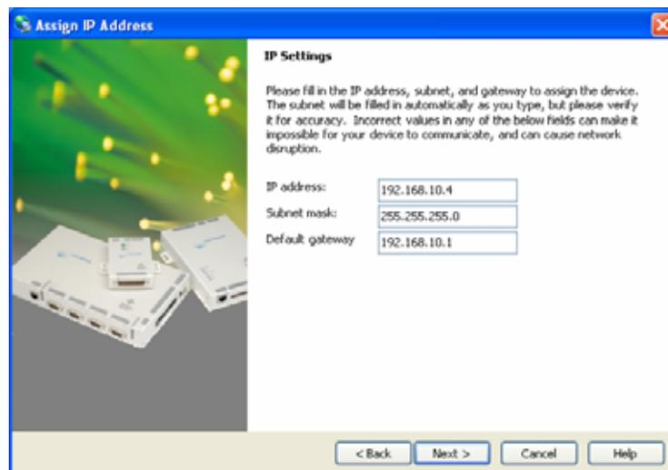
Figure 4-8. Static IP Address Definition
