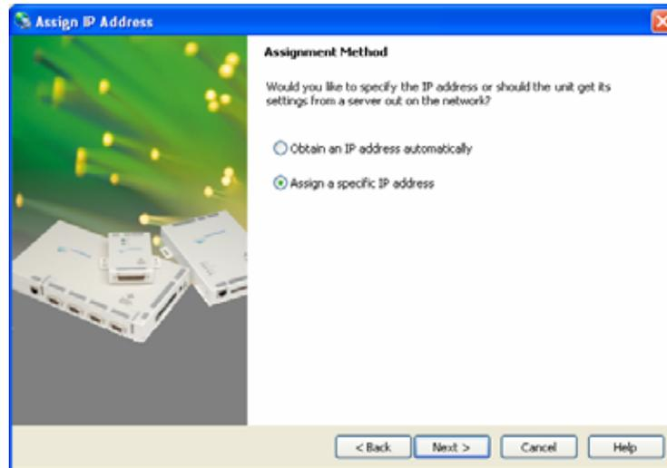
Figure 4-7. Static IP Address
