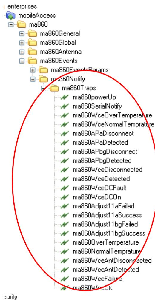
Figure 6-6. MIB Tree with Loaded MobileAccess MA 860
