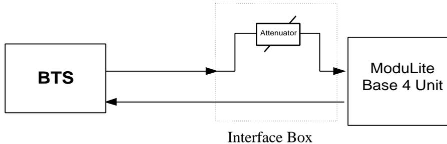
Figure 27: Example - Two port BTS/RBS connected to 1 MBU 4 ports
