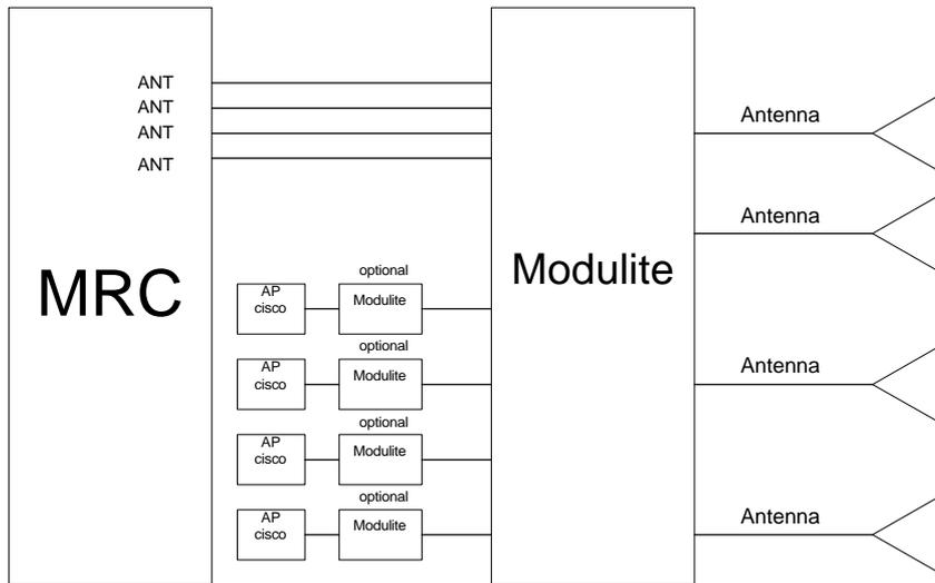
Figure 23 - system configuration with ModuLite 840
