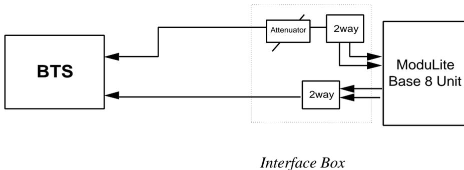
Figure 28: Example- Two port BTS/RBS connected to IMBU 8 ports
