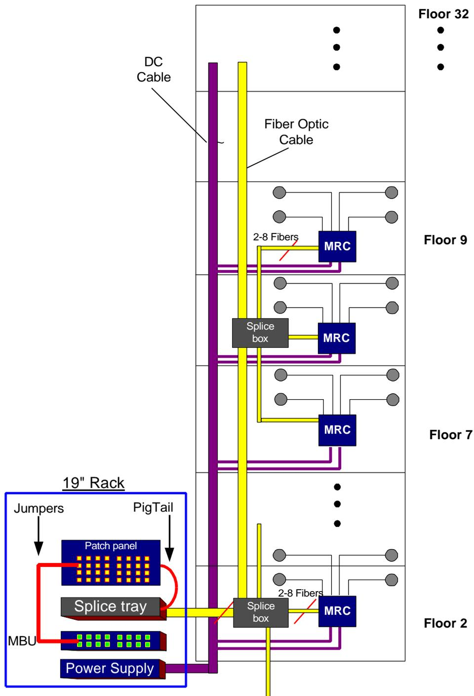
Figure 17: Example - ModuLite™ Installation (fiber and coax)
