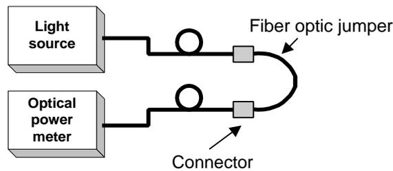
Figure 33: Single Point Test
