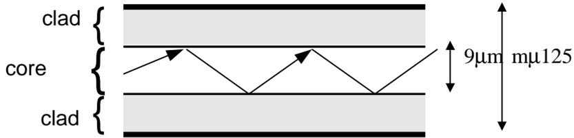
Figure 30: Fiber Optic Cable Structure
