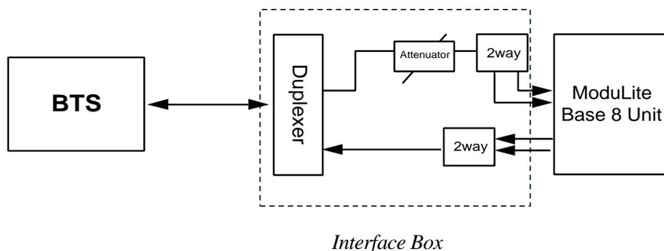
Figure 26: Example - One port BTS/RBS connected to 1 MBU 8 ports
