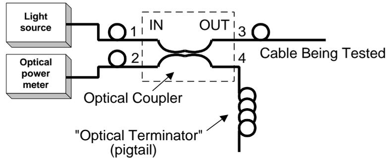
Figure 34: Optical Return Loss Measurement
