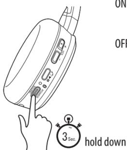
ON : The indicator lights up in blue for 1 second. The indicator flashes slowly in blue when the unit is connected, and flashes slowly in red when the unit is not connected.
