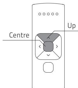
**9.1** Simultaneously hold the **centre** and the **up** button until the blind stops stepping and starts stepping again.
