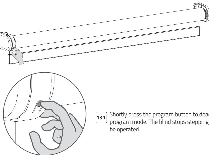
**13.1** Shortly press the program button to deactivate program mode. The blind stops stepping and can be operated.
