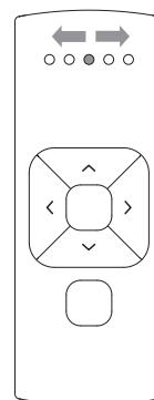
**20.3** Once a blind is found, the channel LED will flash and the blind starts stepping, indicating that program mode has been activated. The blind can now be (un)pai red to the remote and/or programmed.
