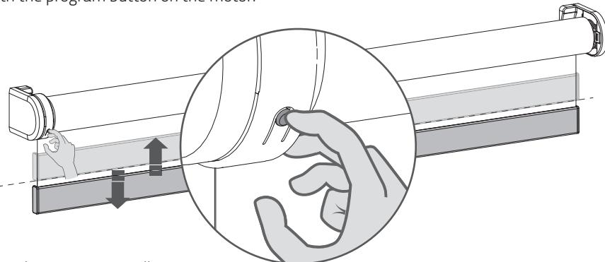
**19.1** Hold the **program** button to manually operate the blind. The blind will move as long as the button is being pressed. (max. 15 sec.)
