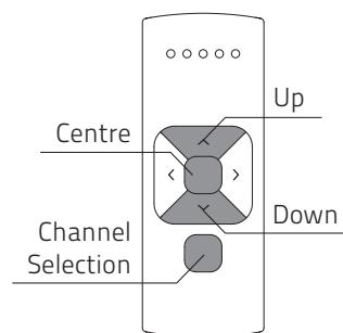
**i** **Remote control:** choose the channel to which the blind has been paired using the **channel** button.
