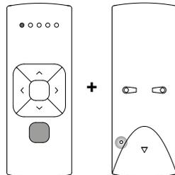
22.3 All blinds in the selected channel will start stepping, indicating program mode has been activated. All blinds can be copied to a new channel on the same remote or other remote. Select a new channel on the (new) remote.
