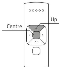
**25.2** Check the direction of rotation of the bottom rail (see step 6) and move the bottom rail to the desired top position. Simultaneously hold the **centre** and the **down** button on the remote until the blind stops stepping and starts stepping again. The top position has been saved
