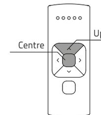
**26.2** Check the direction of rotation of the middle rail (see step 6) and move the bottom rail to the desired top position. Simultaneously hold the **centre** and the **down** button on the remote until the blind stops stepping and starts stepping again. The top position has been saved
