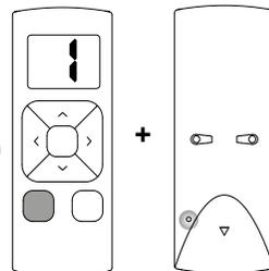
23.3 All blinds in the selected channel will start stepping, indicating program mode has been activated. All blinds can be copied to a new channel on the same remote or to other remotes. Select a channel on a (new) remote.
