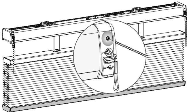
**25.1** Pair the bottom rail motor to an empty channel on the remote. (see step 5)
