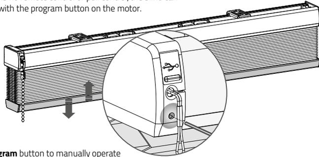
**20.1** Hold the **program** button to manually operate the blind. The blind will move as long as the button is being pressed. (max. 15 sec.)
