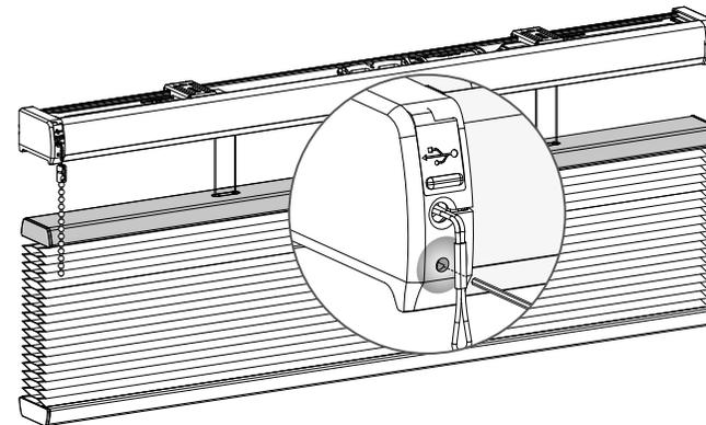
**27.1** Pair the middle rail motor to an empty channel on the remote. (see step 5)
