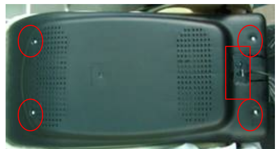
Using the plus screwdriver screw off 8pcs screws
