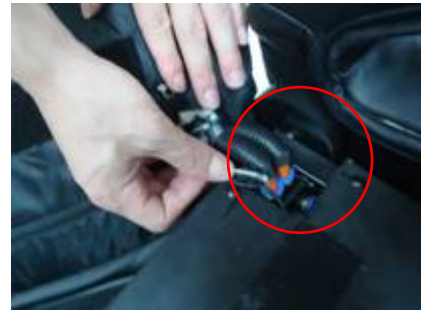
Connector of air hose and motor wires
