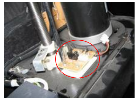
Terminal of the wire and 3pcs screws
