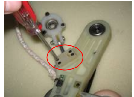
Slacken the screws and take out the ball top of rod
