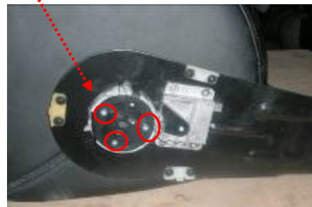
Remove the screw(3pcs) of right side
