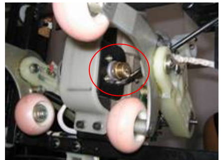
Screw off the tapping motor's screws
