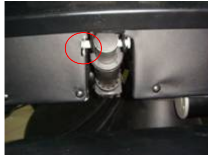
Take off the splint pin Separate the actuator with legrest
