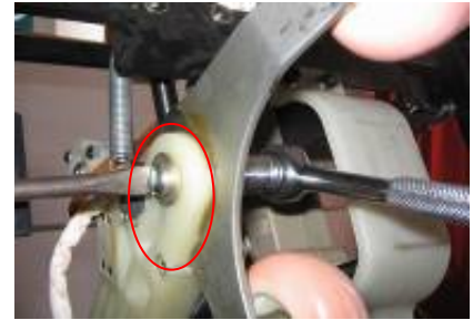
Disassemble the holder of knead balls
