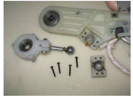
Take off the screws and universal rod
