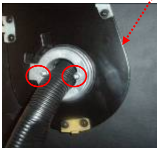
Remove the screws(2pcs) of left side
