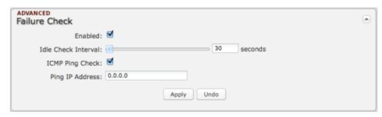
Idle Check Interval: The amount of time between each check. (Default: 30 seconds. Range: 10-3600 seconds.)
