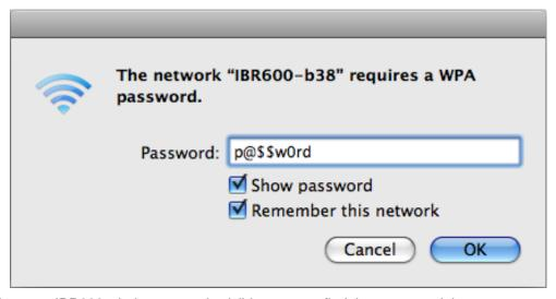
NOTE: If more than one IBR600 wireless router is visible, you can find the correct unit by checking for its **SSID** (service set identifier; the unique name of the local network). The default SSID of the primary network has the form IBR600-xxx, where "xxx" is the last 3 digits of the router's MAC address.
