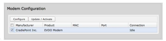
Modem Activation / Update: Activate, Reactivate, or Upgrade Configuration. Click Activate to start the process.
