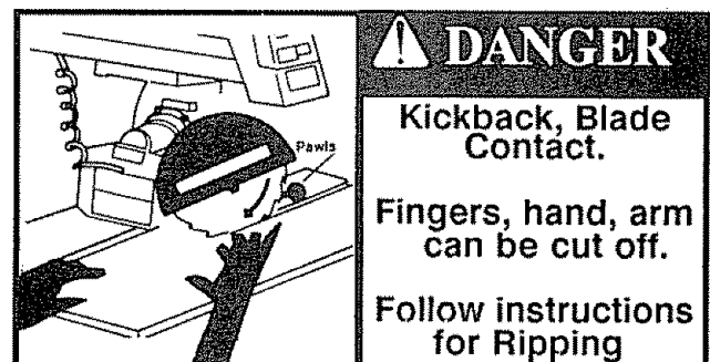
Fig. 3 Blade Contact Safety Sign
