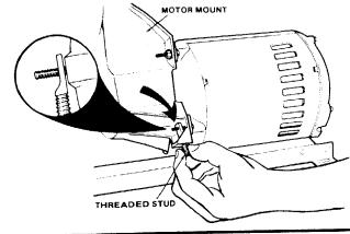
10. Install a flanged lock nut onto this motor stud. Tighten the flanged lock nuts, using a 3/8-inch wrench, until almost tight.
