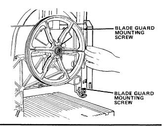
2. Loosen the upper blade guide assembly and lower to approximately 3 inches above rear table and retighten lock knob. This is necessary to make adjustments to blade guide and back up roller bearing.
