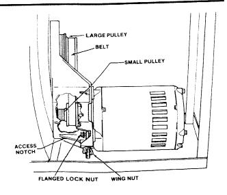
14. Belt tensioning is done by tightening the wing nut which pulls the motor down. The motor slides on the three (3) spacers and is locked in place by the flanged lock nut at the threaded stud.
