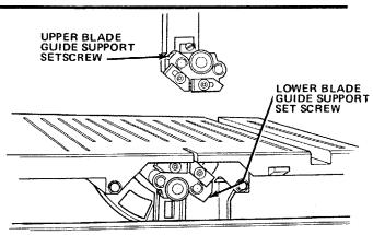
Loosen the setscrew which locks the upper back up bearing and push the bearing all the way back. Repeat procedure for lower back up bearing.
