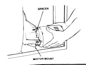
9. Install the threaded stud through the hole in the lower leg of the motor mount and over the motor stud as shown. Install the wing nut onto the threaded stud and turn wing nut until motor slides down tensioning the belt.
