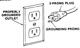
This power tool is equipped with a 3-conductor cord and ground type plug listed by Underwriters' Laboratories. The ground conductor has a green jacket and is attached to the tool housing at one end and to the ground prong in the attachment plug at the other end.
