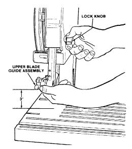
Loosen the two capscrews that lock the upper blade guides using a 1/8-inch hex "L" wrench and separate them about 1/8-inch. Repeat the same step for the lower blade guides.
