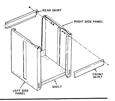
Secure rear of shelf to right side and left side panels using two (2) 1/4-20 x 1/2 truss head bolts, lockwashers, and hex nuts. Hand tighten nuts only at this time.
