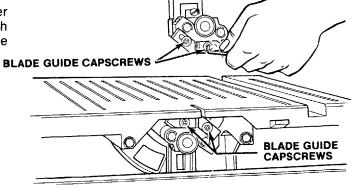
4. Loosen the setscrew which locks the blade guide support and push the support all the way back. Repeat for lower blade guide support.
