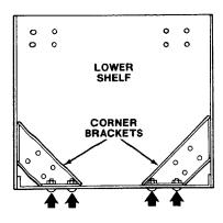
4. Locate the two (2) side panels, one (1) shelf stiffener, and six (6) 1/4-20 x 1/2 truss head bolts, lockwashers and hex nuts. Place the right side panel on its back side as illustrated. Stand up the lower shelf on the rear flange and line up the holes on the corner bracket and shelf stiffener with the holes in the side panel. Mount the bolts in the three holes and tighten hex nuts with a 7/16-inch wrench or socket. Repeat procedure for left side panel.
