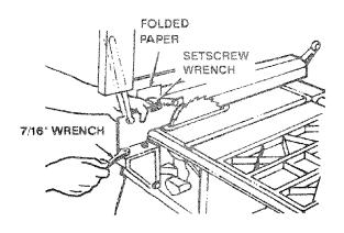
21. To remove BLADE GUARD AND SPREADER, loosen THUMBSCREW...DO NOT LOOSEN OTHER SCREWS. This lets you remove and replace the guard without disturbing the spreader alignment.
