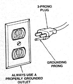
WARNING: To avoid electrical shock, do not permit fingers to touch the terminals of the plug, when installing or removing the plug to or from the outlet.
