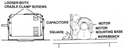
WARNING: Failure to properly install motor may let workpiece strike capacitor cover during bevel or compound miter cuts. Workpiece could bind and kickback. You could be cut or hit.
