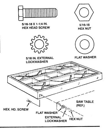
Line up front edge of extension with front edge of table. Link up top surface of extension with top surface of table at the locations indicated by the "X"s (see illustration).
