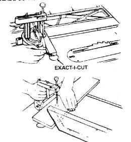
11 MICRO-ADJUST RIP FENCE...allows the operator to accurately adjust the rip fence using only one hand. To move the fence, push in on the micro-adjust knob and rotate the knob. Rotating the knob clockwise moves the fence to the left. Rotating it counterclockwise moves the fence to the right.
