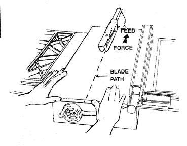
When "WIDTH OF RIP" is 2 in. or wider, USE THE PUSH STICK to finish pushing the work all the way past the blade.
