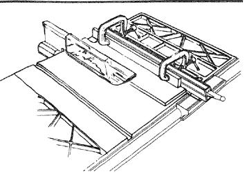
Feed the workpiece by hand along the AUXILIARY FENCE until the end is approx. 1 in. past the front edge of the table. Continue to feed using the PUSH BLOCK.
