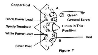
c. Replace the 120v power cord plug with a (3 blade) 240v 15 Amp U.L. listed plug (see illustration below). Connect the power cord white and black leads, respectively, to the two "hot" plug blades and connect the power cord grounding wire to the plug ground prong.
