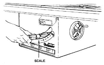
If blade is NOT 45° TO TABLE...STOP SCREW and SCALE must be ADJUSTED.
