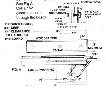
6 MITER GAUGE...head is locked in position for crosscutting or mitering by tightening the lock knob. ALWAYS LOCK IT SECURELY WHEN IN USE. There are slots for the stop pin at the 45 degree right and left positions for conveniently setting the Miter Gauge to cut miters.
