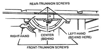
8. Using a wood block and mallet as shown, move rear trunnion to right or left as required to realign the blade. If necessary, shift front trunnion in similar manner; but do NOT move front trunnion unless necessary. Recheck the alignment with the square, then securely retighten all six trunnion screws.
