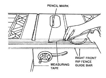
**NOTE:** If extreme accuracy is required when ripping, you should not use this method to position the fence. Instead, use a precision measuring instrument to set the rip fence the exact distance away from the blade.
