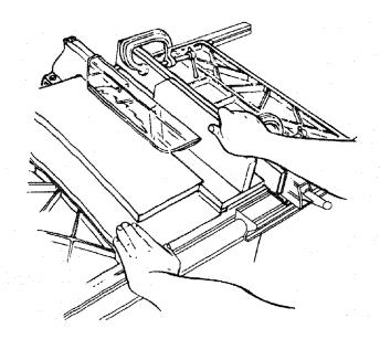
Narrow strips thicker than the Auxiliary Fence/Work Support may enter the guard and strike the baffle. CAREFULLY raise guard only enough to clear the workpiece. Use PUSH BLOCK to complete cut.
