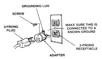
This plug requires a mating 3-conductor grounded type outlet as shown above.
