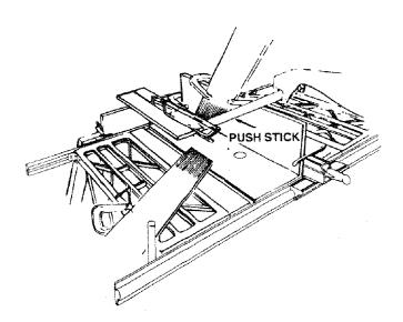
WARNING: To avoid kickback push forward only on the part of the workpiece that will pass between the blade and the fence.
