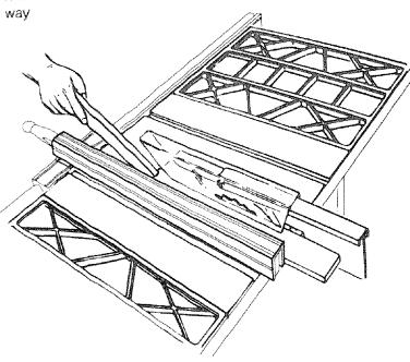
When WIDTH OF RIP is 1/2" to 2 in., the push stick CANNOT be used because the guard will interfere. USE the AUXILIARY FENCE/WORK SUPPORT and PUSH BLOCK.
