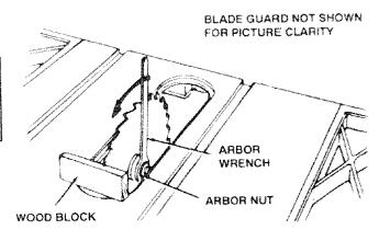
When installing the blade, make sure the teeth are pointing toward the front of the saw and that the blade and collars are clean, and free from any burrs. The HOLLOW side of the collar must be against the blade. Always tighten the arbor nut securely.
