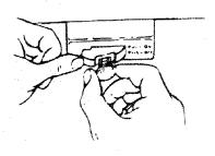
2 ELEVATION HANDWHEEL...elevates or lowers the blade. Turn clockwise to elevate...counterclockwise to lower.
