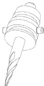
FIGURE 5: 1/16" CARVING BIT WITH ADAPTER
