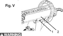
To avoid injury from materials being thrown, always unplug the saw to avoid accidental starting, and remove small pieces of material from the table cavity. The table insert may be removed for this purpose, but always reattach the table insert prior to performing a cutting operation.
