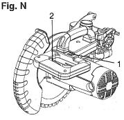
Your tool is equipped with the Laser Trac® cutting guide using a Class Illa laser beam. The laser beam allows you to preview the saw blade path on the stock to be cut before starting the miter saw. This laser guide is powered by the transformed alternating current supply directly through the power lead. The saw must be connected to the power source and the laser on/off switch must be turned on for the laser line to show.
