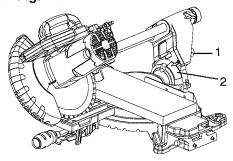
**NOTE:** The saw comes with a 33.9° crown molding stop.
