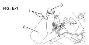
REMOVING OR INSTALLING THE BLADE
