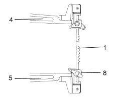
Tilt the table to a 45° angle and lock the bevel lock knob to view lower blade holder (8). (Fig. J) NOTE: Apply slight downward pressure on the upper arm when removing the blade from the upper blade holder.
