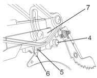
Removing the blade guard and antikickback pawl assembly (Fig. R, T-1)
