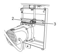
**NOTE:** If excessive looseness is observed in any part of the blade raising mechanism or tilting mechanism, take the complete unit to a Service Center.
