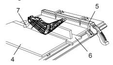
8. Continue pushing the workpiece (4) with the push stick (3) or push block (6 - Fig. YY) until it passes through the blade guard and clears the rear of the table. (Fig. XX)
