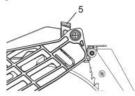
Removing the blade guard and antikickback pawls assembly (Fig. X, AA)
