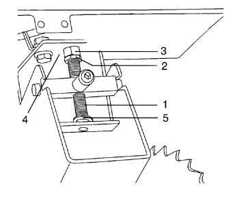
You can place a small amount of dry lubricant on bevel andgle adjustment rod also. This rod (1) must be kept clean and free of sawdust, gum, pitch, and other contaminants for smooth operation.
