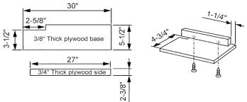
Attach auxiliary fence to rip fence with two "C" clamps. (Fig. CC-2)
