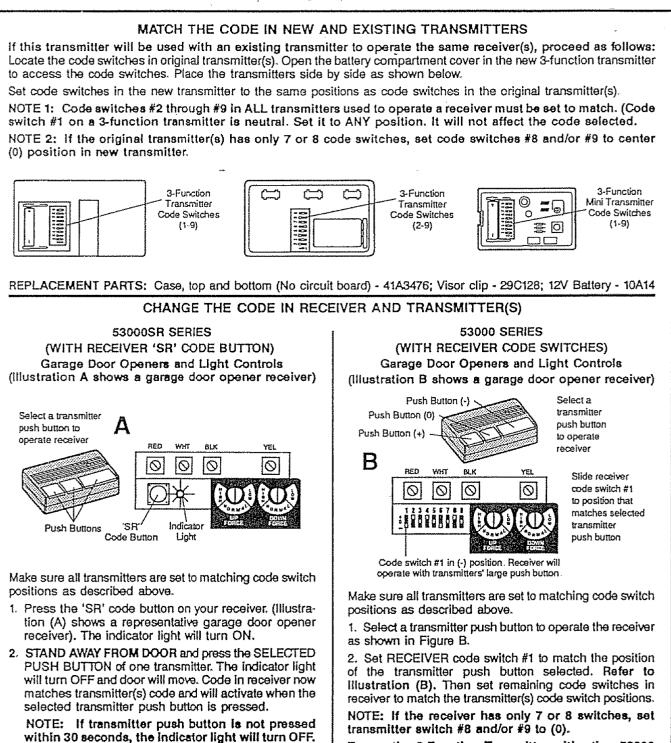
To use the 3-Function Transmitter with other 53000 Series receivers: Set receiver code switch #1 to match the position of another transmitter push button. Then set remaining code switches to match transmitter(s) code switches.
