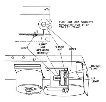
CAUTION: If the door opener is installed on a door with a height greater than 6 feet, the "UP" limit must be adjusted.
