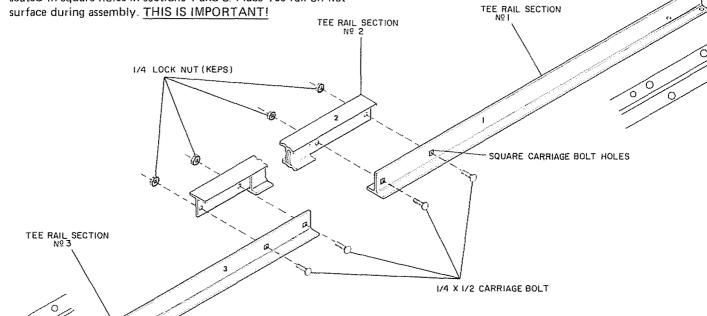
Bolt section 1 to section 2. Use 1/4 inch by 1/2 inch carriage bolts, and 1/4 inch lock nuts.
