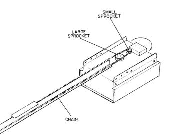
CAUTION: The chain retainer bracket should be kept in the illustrated position during assembly.
