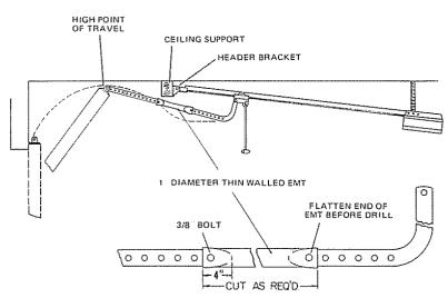
REMOTE INSTALLATION PROCEDURES: (1) Fasten header bracket to a suitable support on ceiling (a 2x4 or 2x6 reinforcing plank nailed to joists, for example). The support location should be the most convenient in line with the door bracket and further inside the garage than the highest point of door travel.
