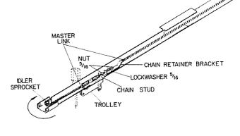
Connect the chain to the chain retainer bracket using the second master link in the coin envelope. Slide the chain retainer bracket onto the chain stud as illustrated. Secure it to the stud with the second 5/16 inch nut and lock washer.
