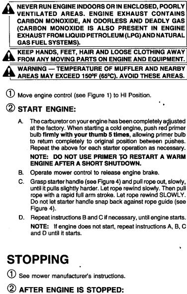
A. DISCONNECT SPARK PLUG WIRE FROM SPARK PLUG AND ATTACH IT TO RETAINING POST (see Figure 6).
