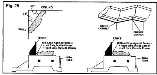
Crown Molding Flat on Miter Table
