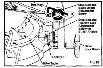
⚠ WARNING: DO NOT start your compound miter saw without checking for interference between the blade and the miter table support. The blade could be damaged if it strikes the miter table support during operation of the saw.
