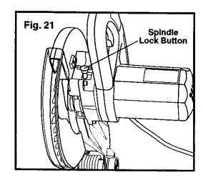
⚠ WARNING: To prevent damage to the spindle lock, ALWAYS allow the motor to come to a complete stop before engaging the spindle lock. ALWAYS make sure the spindle lock is disengaged before reconnecting saw to the power source.
