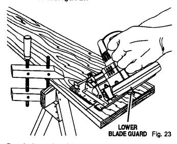
Rest the front edge of the base on the workpiece. Depress the lock-off button and squeeze the switch trigger to start your saw. **Always** let the blade reach full speed, then guide your saw into the workpiece.
