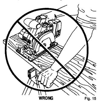
Never place your hand on the workpiece behind your saw while making a cut.
