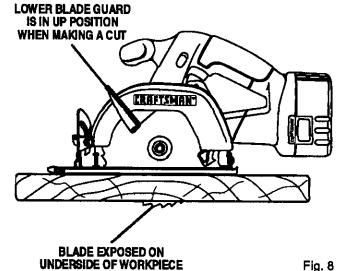
Never use saw when guard is not operating correctly. Guard should be checked for correct operation before each use. If you drop your saw, check the lower blade guard and bumper for damage at all depth settings before reuse. Note: The guard is operating correctly when it moves freely and readily returns to the closed position. If for any reason your lower blade guard does not close freely, take it to the nearest Sears Parts and Repair Center for service before using.
