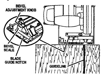
ALIGN INNER BLADE GUIDE NOTCH ON SAW BASE WITH LINE OF CUT AS SHOWN WHEN MAKING 45° BEVEL CUTS Align your line of cut with the inner blade guide notch on the saw base when making 45° bevel cuts.
