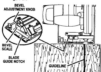
ALIGN INNER BLADE GUIDE NOTCH ON SAW BASE WITH LINE OF CUT AS SHOWN WHEN MAKING 45° BEVEL CUTS Align your line of cut with the inner blade guide notch on the saw base when making 45° bevel cuts.
