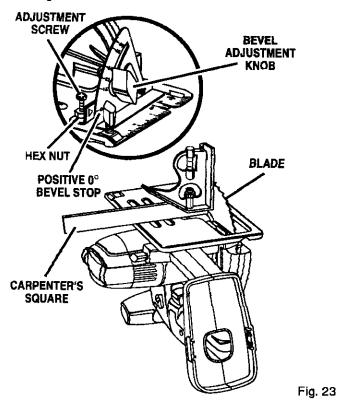
Your saw has a positive 0° bevel stop, that has been factory adjusted to assure 0° angle of your saw blade when making 90° cuts. However, misalignment can occur during shipping.
