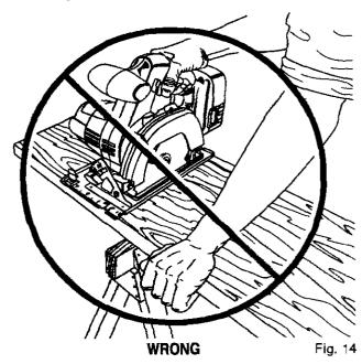
Never place your hand on the workpiece behind your saw while making a cut.
