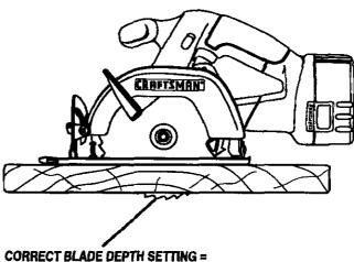
**BLADE EXPOSED ONE BLADE TOOTH BELOW THE MATERIAL TO BE CUT**
