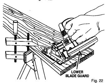
Rest the front edge of the base on the workpiece. Depress the lock-off button and squeeze the switch trigger to start your saw. **Always** let the blade reach full speed, then guide your saw into the workpiece.
