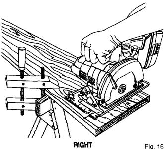
Depress the lock-off button and squeeze the switch trigger to start your saw. **Always** let the blade reach full speed, then guide your saw into the workpiece.
