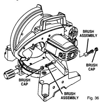
Your saw has externally accessible brush assemblies that should be periodically checked for wear.
