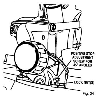
Retighten bevel lock knob. Next, retighten lock nut securing the positive stop adjustment screw.
