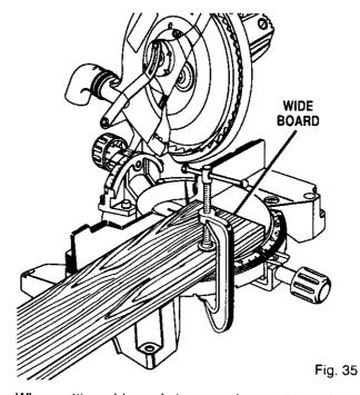
When cutting wide workpieces such as a 2 in. x 6 in., boards should be clamped with a C-clamp as shown in figure 35.
