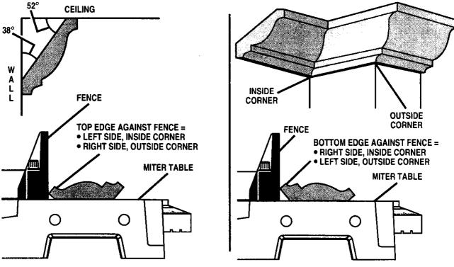
**CROWN MOLDING FLAT ON MITER TABLE**
