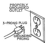
This tool is intended for use on a circuit having a nominal rating less than 150 volts which has an outlet that looks like the one illustrated above.
