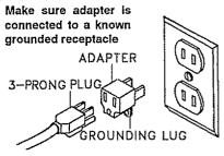
NOTE: The adapter illustrated is for use only if you already have a properly grounded 2-prong receptacle. Adapter is not allowed in Canada by the Canadian Electrical Code.
