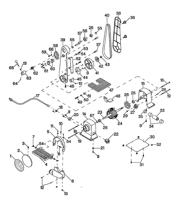
Figure 4—Replacement Parts Illustration
