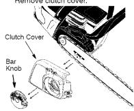
Slide guide bar on bar bolts until guide bar stops against clutch drum sprocket.
