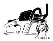
3. Turn adjusting wheel (downward direction) to tension chain until chain solidly contacts bottom of guide bar rail. Lift tip of guide bar while adjusting tension.
