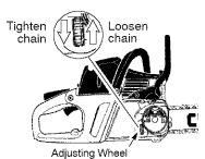
4. Using screwdriver, move chain around guide bar to ensure all links are in bar groove.
