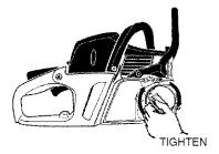
6. Push lever on bar knob down to return lever to closed/locked position.
