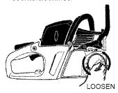
Loosen chain tension by turning adjusting wheel (upward direction). Remove clutch cover.
