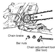
Turn adjusting screw on bar counterclockwise to move the tensioning rack as far as it will go toward the front of the bar.
